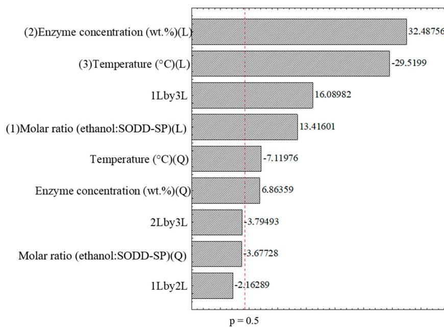
**Figure A2.** Pareto chart with the effects of the parameters and their interactions for the experimental design of the esterification/transesterification with SODD saponifiable phase and ethanol using Eversa Transform 2.0 as biocatalyst.
