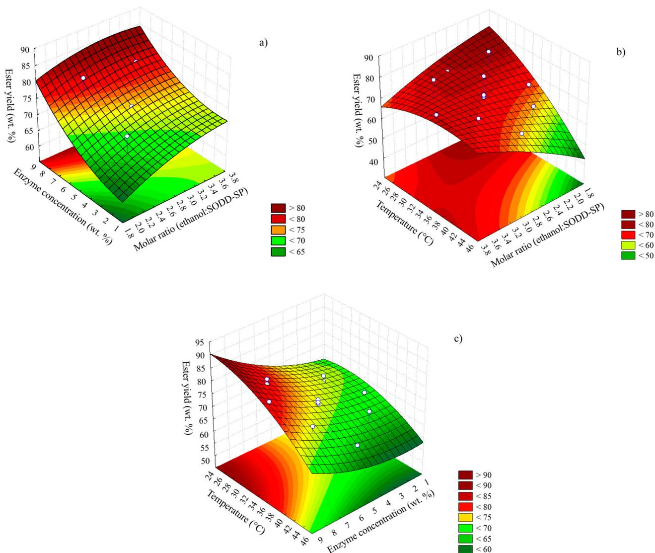
**Figure 2.** Response surfaces of biodiesel reaction with SODD saponifiable phase (SODD-SP). (a) Enzyme concentration vs. ethanol:SODD-SP molar ratio. (b) Temperature vs. ethanol:SODD-SP molar ratio. (c) Temperature vs. enzyme concentration. Z-axis indicates the ester yield (wt. %).
