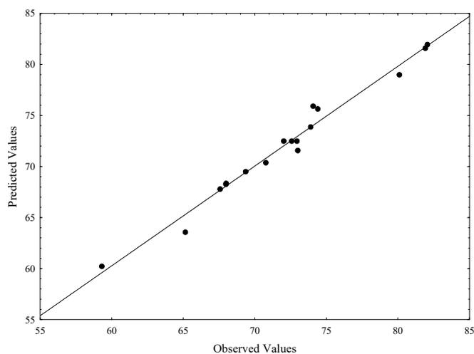
**Figure A1.** Correlation between experimental (**observed values**) and fitted (**predicted values**) ester yields (wt.%) of the esterification/transesterification with SODD saponifiable phase and ethanol using Eversa Transform 2.0 as biocatalyst.
