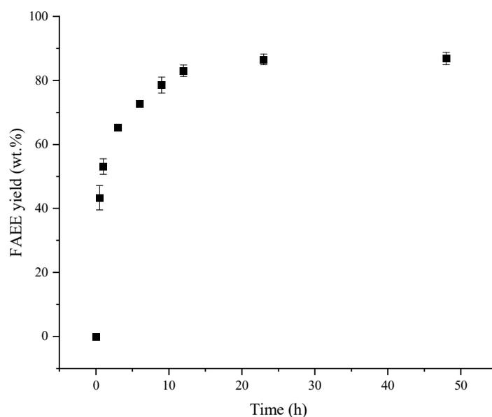
**Figure 3.** Profile of fatty acid ethyl ester (FAEE) yield (wt.%) vs. time for the esterification/transesterification of SODD saponifiable phase (SODD-SP) (15 g) with ethanol (8.10 g). Reactions conditions: up to 48 h reaction; 35 °C; molar ratio of 3.64:1 (ethanol:SODD-SP) and 8.36 wt.% enzyme concentration.
