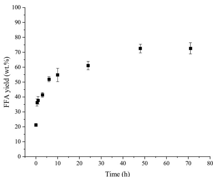
**Figure 1.** Free fatty acid (FFA) yield profile (wt.%) vs. time for the hydrolysis of SODD by the enzyme Eversa Transform 2.0. Reaction conditions: up to 72 h reaction; 37 °C; 4:1 mass ratio (H<sub>2</sub>O:SODD) and 5% enzyme (m/mSODD).
