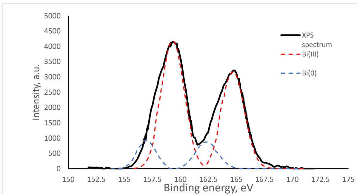
Figure 5. XPS spectrum of sample 2.
