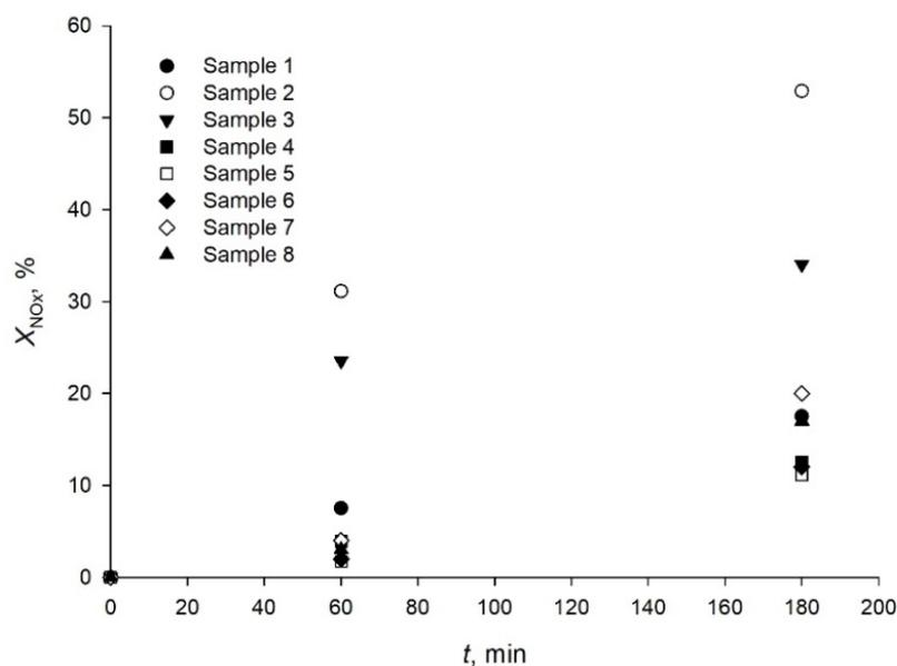
Figure 6. NO<sub>x</sub> degradation for sample 1–8 versus time.
