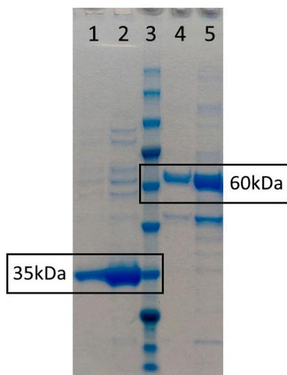
**Figure S12.** SDS/PAGE analysis of purified Fe-P (lane 1-2) and  $\alpha$ L158C MoFe-P (lane 3-4) using FPLC system, molecular weight ladder (Lane 3).
