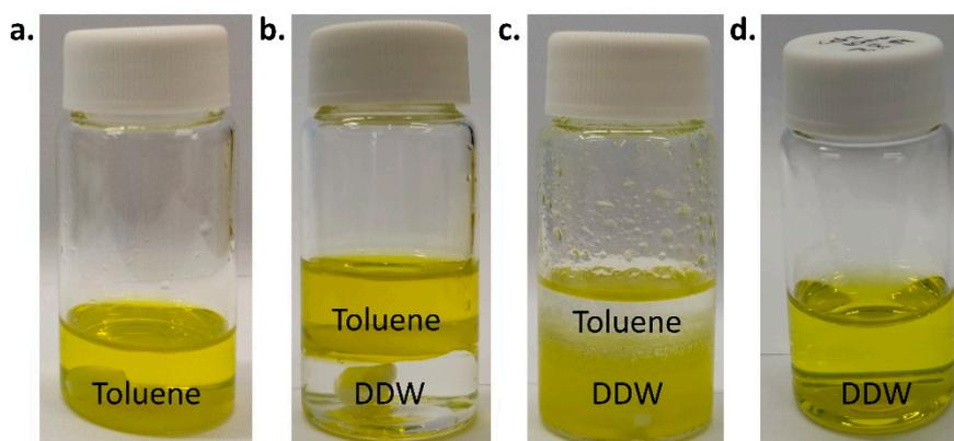
**Figure S2.** CdS Ligand Exchange to ME (a) CdS-OA NPs in Toluene, (b,c) Biphasic mixtures of Toluene and DDW before stirring (b) after stirring (c), d. CdS-ME NPs in DDW after filtration.
