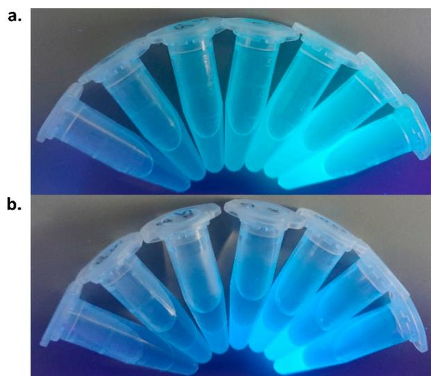
**Figure S7.** Fluorescence emission of calibration curve samples ( $\text{NH}_4\text{Cl}$ ) after derivatization with OPA.
