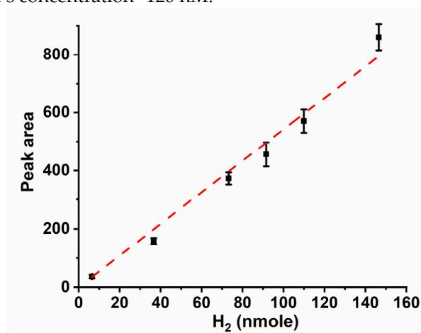
**Figure S5.** Calibration curve for H<sub>2</sub> using GC-TCD. (slope-  $5.4 \pm 0.2$ , R-Square- 0.994)
