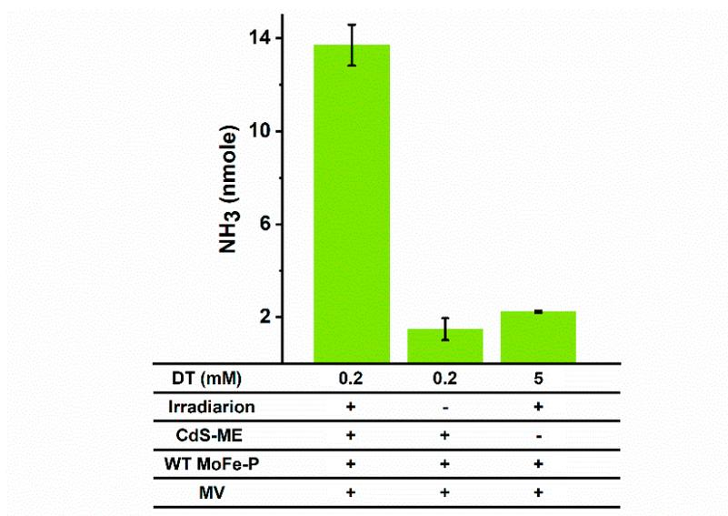
**Figure S10.**  $\text{NH}_3$  production of WT MoFe-P activation by chemically reduced MV with Sodium dithionite (DT, with no CdS NPs) compared to CdS-ME NPs: WT MoFe-P biohybrid systems after 2 hr of irradiation and the same biohybrid system in dark condition as a control.
