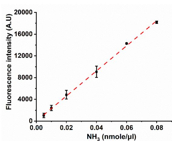
**Figure S6.** Calibration curve for NH<sub>4</sub>Cl using OPA fluorescence assay after extraction to chloroform. (slope-  $231000 \pm 2000$ , R-Square- 0.999)
