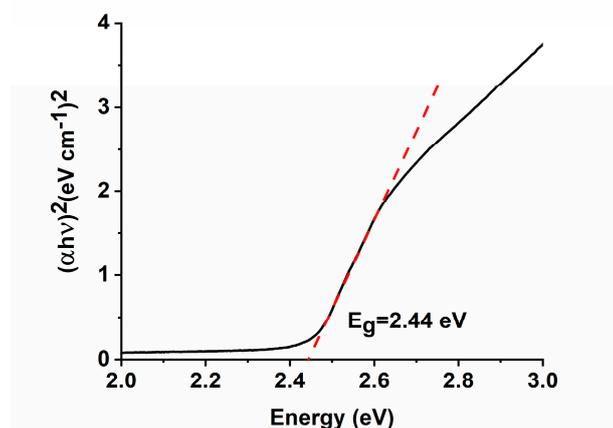
**Figure S4.** Tauc plot of the CdS NPs.
