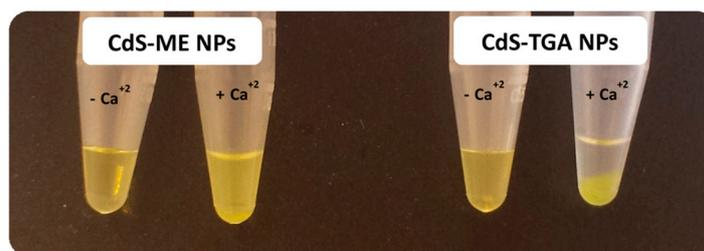
**Figure S3.** CdS-ME and Cd-TGA in the presence of positively charged divalent ions (Calcium ions), aggregation, and sedimentation were observed due to electrostatic crosslinking in the case of CdS-TGA NPs with the presence of calcium ions interaction.
