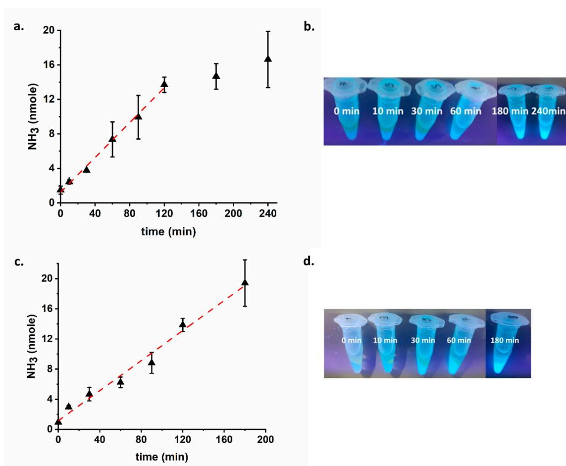
**Figure S9.** (a,c) kinetics of  $\text{NH}_3$  production of mediated CdS-ME NPs: MoFe-P biohybrid systems, (a) WT MoFe-P and (c)  $\alpha$ L158C MoFe-P. (b,d)  $\text{NH}_3/\text{OPA}$  complex's fluorescence emission after extraction to Chloroform of different irradiation time points of mediated CdS-ME NPs: MoFe-P biohybrid systems, (b) WT MoFe-P and (d)  $\alpha$ L158C MoFe-P.
