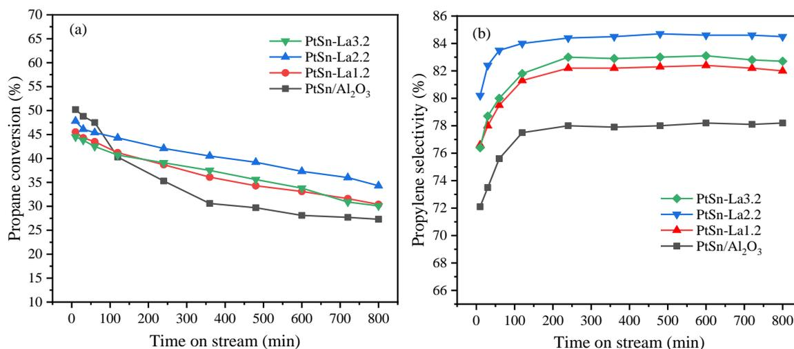
Figure 6. Catalytic performance of the parent  $\text{PtSn}/\gamma\text{-Al}_2\text{O}_3$  catalyst and  $\text{PtSn-LaX}$  catalysts in PDH reaction. (a) Propane conversions with time on stream. (b) Propylene selectivities with time on stream.
