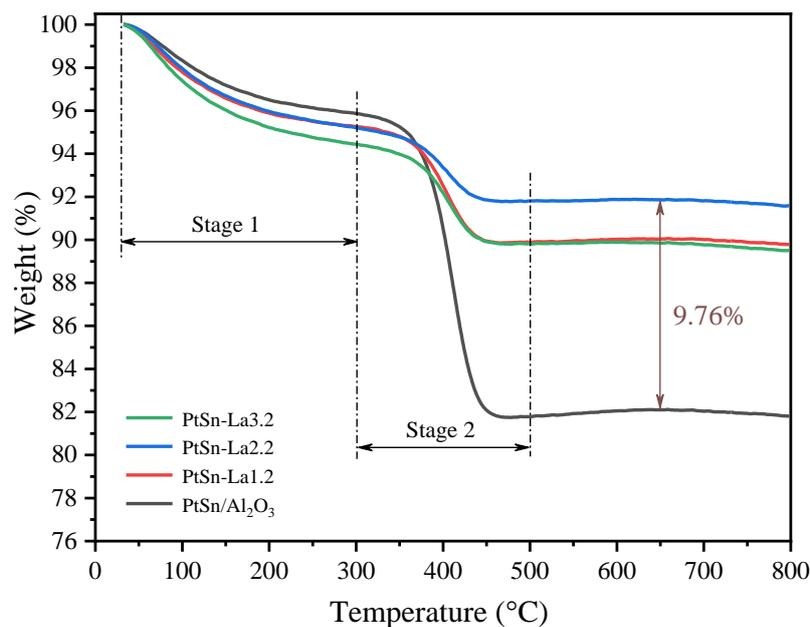
Figure 7. The thermogravimetric (TG) curves of the spent catalysts.
