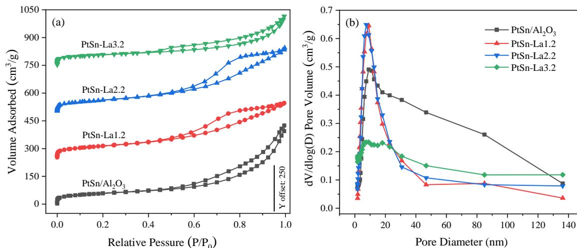
**Figure 2.** Low-temperature N<sub>2</sub> adsorption–desorption isotherms (a) and the corresponding pore size distributions (b) of the parent PtSn/ $\gamma$ -Al<sub>2</sub>O<sub>3</sub> and PtSn-LaX catalysts.
