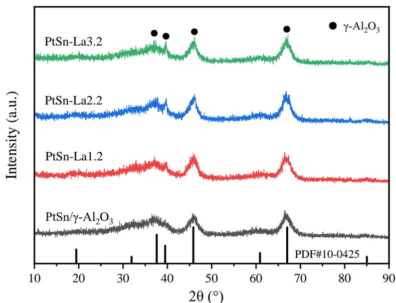
**Figure 1.** XRD patterns of the parent PtSn/γ-Al<sub>2</sub>O<sub>3</sub> catalyst and PtSn-LaX catalysts.
