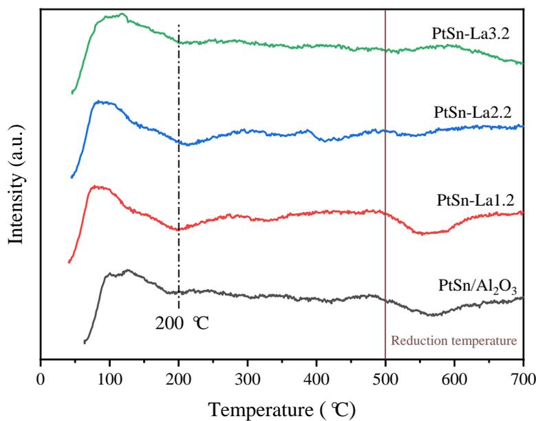
**Figure 4.** The H<sub>2</sub>-TPR profiles of the parent PtSn/ $\gamma$ -Al<sub>2</sub>O<sub>3</sub> and PtSn-LaX catalysts.
