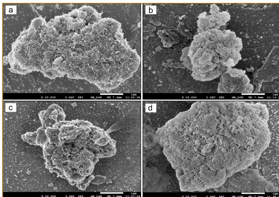
**Figure 3.** SEM images of the parent PtSn/ $\gamma$ -Al<sub>2</sub>O<sub>3</sub> and PtSn-LaX catalysts. (a) PtSn/ $\gamma$ -Al<sub>2</sub>O<sub>3</sub>; (b) PtSn-La1.2; (c) PtSn-La2.2; (d) PtSn-La3.2.
