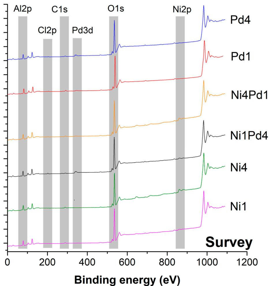
Figure S3. Wide scan survey XPS spectra of the mono and bimetallic catalysts.
