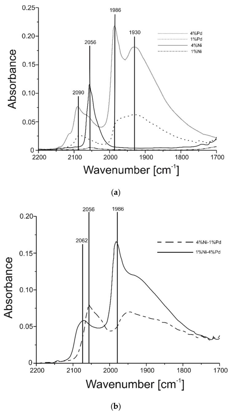
**Figure S4.** FTIR spectra of CO adsorbed on the surface of (a) the monometallic and (b) the bimetallic catalysts recorded after CO evacuation.
