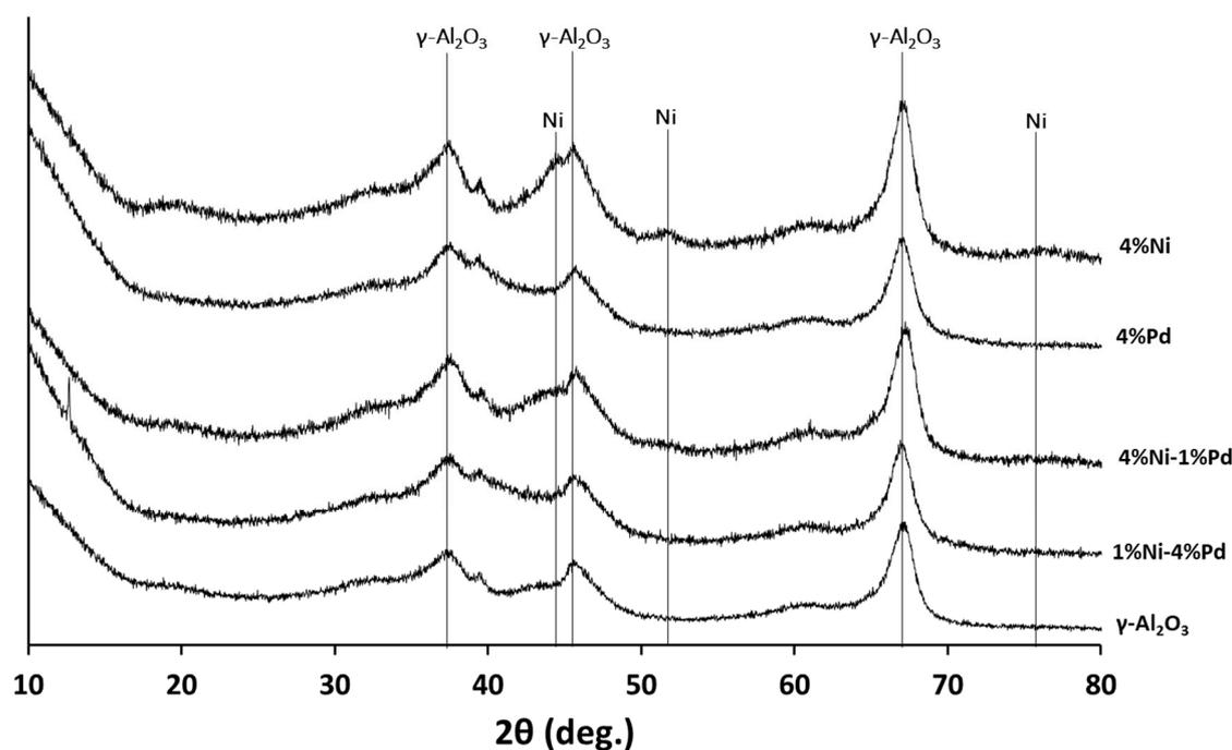
Figure S1. XRD patterns of mono- and bi-metallic catalysts.
