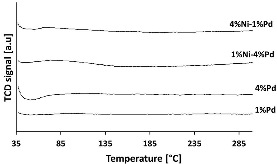
Figure S2. TPR profiles of the mono- and bi-metallic catalysts after the reduction step.
