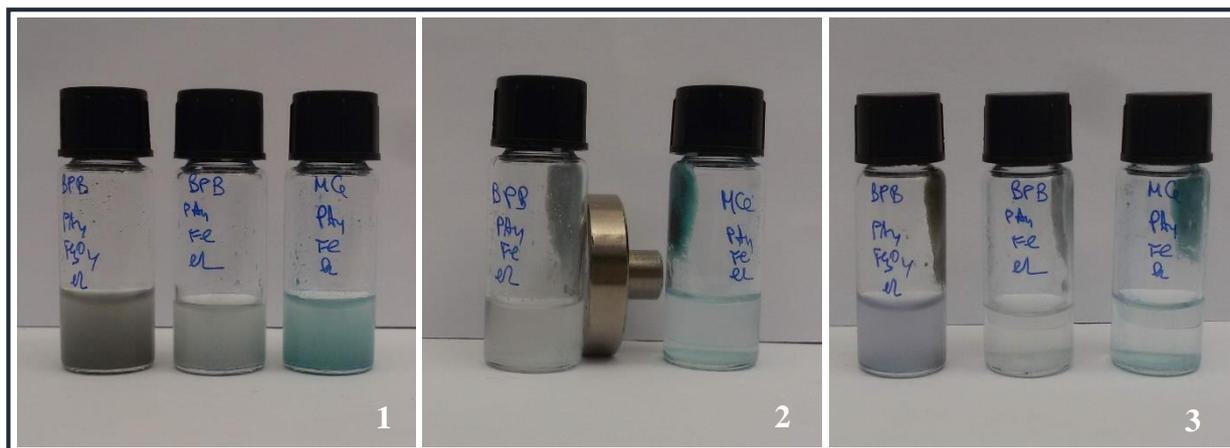
**Figure S5.** | PA4-Fe-eL sample fast removal from DDW suspension: 1 – Conjugate suspension in water; 2, 3 - phases of conjugate separation applying a constant magnet (BPB-bromphenol blue; MG-malachite green).
