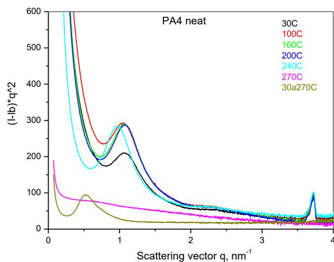
**Figure S3.** Disappearance of the scattering peak at  $q = 3.73 \text{ nm}^{-1}$  in the SAXS patterns after melting and recrystallization of PA4 MP support – see the curves at 270C and 30a270C.
