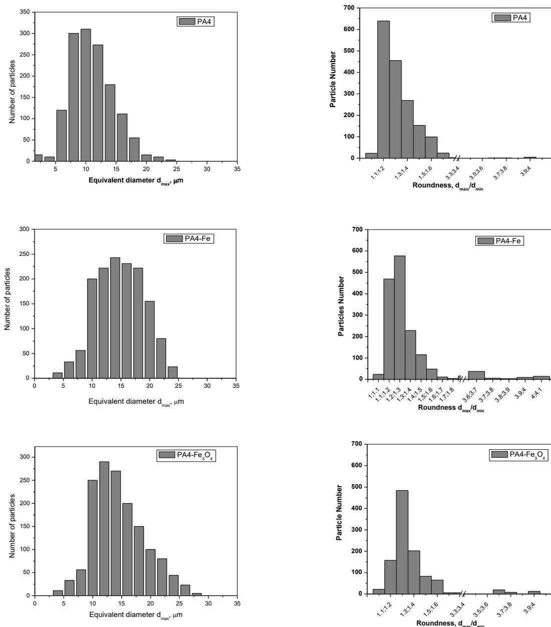
**Figure S2.** Histograms of the average size ( $d_{max}$ ) and roundness ( $d_{max}/d_{min}$ ) distributions for PA4 MP supports based on optical microscopy.
