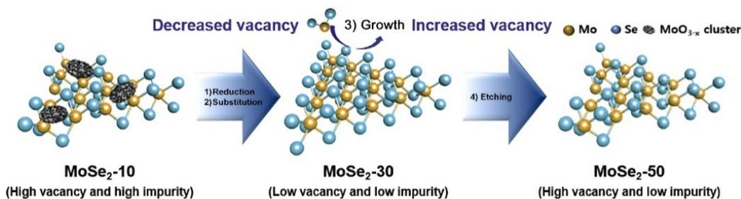
**Scheme 7.** Schematic illustration for growth and synthesize Se-vacancy controlled MoSe<sub>2</sub> with H<sub>2</sub> concentration control. H<sub>2</sub> plays a dual role in enhancing the reduction of MoO<sub>3</sub> (decreased vacancies) and Se etching at the MoSe<sub>2</sub> lattice (decreased vacancies). Reproduced and adapted from Ref. [79]; Copyright (2019), Elsevier.
