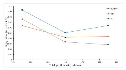
**Figure 5.** Effect of total gas flow rate on the overall mass transfer coefficient in the packed column. The experimental conditions were: liquid temperature of 30  $^{\circ}$ C, absorbent concentration of 10 wt.%, inlet CO<sub>2</sub> concentration of 20 vol.% and a liquid flow rate of 4 mL/min.
