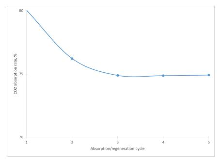
Figure 9. Absorption/regeneration behavior for aqueous absorbent [TBP][Lys] at 10 wt%.
