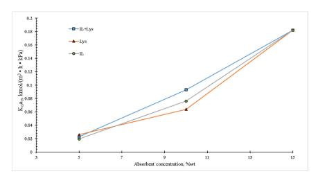
**Figure 7.** Effect of the absorbent concentration on the overall mass transfer coefficient in the packed column. The experimental conditions were: liquid temperature of 30  $^{\circ}$ C, inlet CO<sub>2</sub> concentration of 20 vol.% and total gas and liquid flow rates of 100 and 4 mL/min, respectively.
