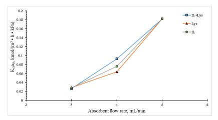
**Figure 6.** Effect of the liquid flow rate on the overall mass transfer coefficient in the packed column. The experimental conditions were: liquid temperature of 30 °C, absorbent concentration of 10 wt.%, inlet CO<sub>2</sub> concentration of 20 vol.% and gas flow rate of 100 mL/min.
