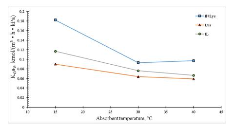
**Figure 8.** Effect of the absorbent temperature on the overall mass transfer coefficient in the packed column. The experimental conditions were: inlet CO<sub>2</sub> concentration of 20 vol.%, liquid concentration of 10 wt.% and total gas and liquid flow rates of 100 and 4 mL/min, respectively.
