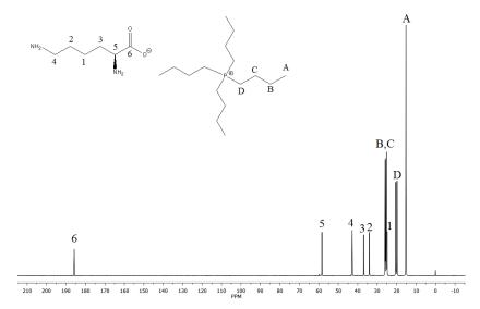
**Figure 2.** <sup>13</sup>C NMR spectrum of tetrabutylphosphonium lysinate. Signal **A** corresponds to carbon atom in final position of butyl group. Signal **B**, **C** and **D** corresponds to carbons with double signal C-P.
