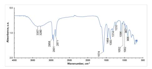
**Figure 3.** FTIR spectrum of tetrabutylphosphonium lysinate.
