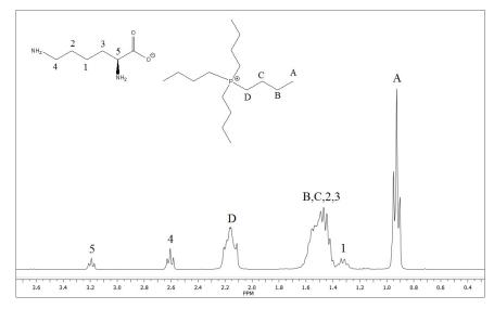
**Figure 1.** <sup>1</sup>H NMR spectrum of tetrabutylphosphonium lysinate. Signal **A** corresponds to hydrogens atoms from methyl group of n-butyl, signals **B** and **C** corresponds to multiplet from intermediate methyl groups and **D** corresponds to hydrogen atoms from methyl group next to phosphorus atom.
