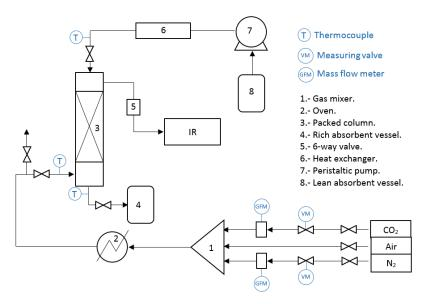
Figure 10. Continuous CO<sub>2</sub> absorption system.
