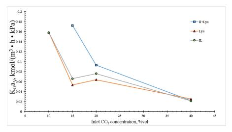
**Figure 4.** Effect of inlet  $CO_2$  concentration on the overall mass transfer coefficient in the packed column. The experimental conditions were: liquid temperature of 30 °C, absorbent concentration of 10 wt.% and the total gas and liquid flow rates of 100 and 4 mL/min, respectively.
