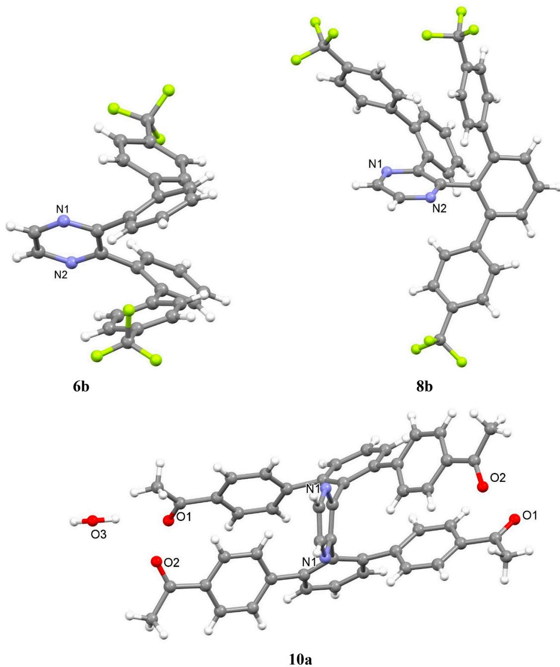
**Figure S2:** Crystal structures of **6b**, **8b** and **10a**. Disorder on CF<sub>3</sub> groups in **6b** and **8b** has been omitted for clarity. Asymmetric unit of **10a** is composed of a half of molecule **10a** and a half of water molecule.
