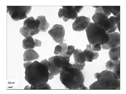
**Figure S1.** TEM micrograph of AuZ catalyst
