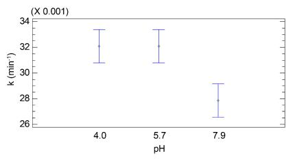
Figure S4. Statistical analysis of the effect of the pH value on the pseudo-first order rate constant of the photocatalytic degradation meropenem
