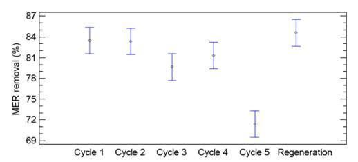
**Figure S5.** Statistical analysis of the effect of the reuse of the  $TiO_2$ /fiberglass substrate on the removal of MER after 60 min of reaction (pH = 5.7)
