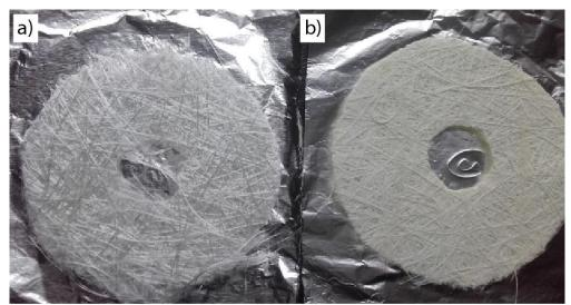
Figure S1. a) Fiberglass disc before immobilization b) TiO<sub>2</sub>/fiberglass substrate
