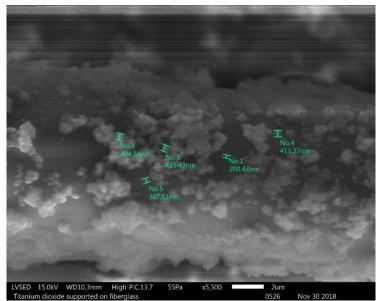
**Figure S2.** SEM images of the TiO<sub>2</sub>/fiberglass substrate. The size of some agglomerates of TiO<sub>2</sub> immobilized on fiberglass is reported
