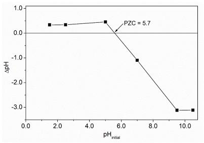
Figure S3. Point of zero charge of the TiO<sub>2</sub>/fiberglass substrate
