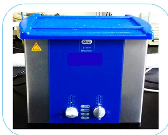
**Figure 9.** The ultrasonication instrument for the extraction of the original DCLR.
