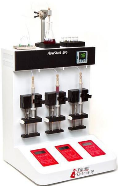
**Figure S85.** Instrument used for the C-H  $^{18}\text{F}$ -difluoromethylation reaction of the heteroarenes (FlowStart Evo, FutureChemistry).
