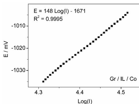
**Figure 7.** Tafel slope for the Gr/IL/Co system measured in the phosphate buffer pH = 7, Ω = 5 mV·s<sup>−1</sup>.
