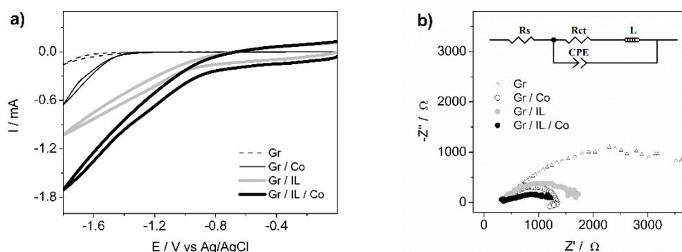
**Figure 5.** (a) Voltammetric profiles and (b) Nyquist plot towards a hydrogen evolution reaction (HER) and equivalent circuit used. Phosphate buffer at pH = 7, in Ar saturation.  $\Omega = 0.1 \text{ V}\cdot\text{s}^{-1}$ .
