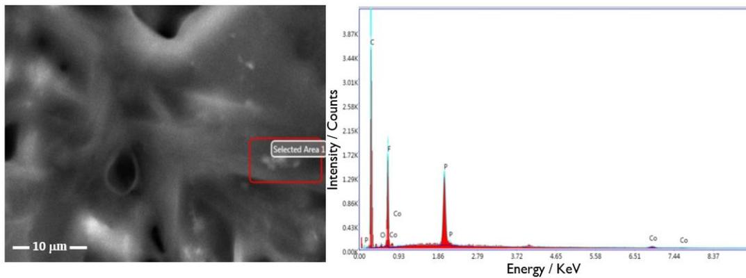
**Figure 3.** FESEM image and composition study by EDX for the system Gr/IL/Co. Magnification = 6525 $\times$ .
