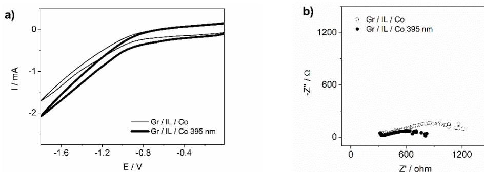
**Figure 6.** (a) Voltammetric profiles and (b) Nyquist plot towards HER. Phosphate buffer at pH = 7 in Ar saturation.  $\Omega = 0.1 \text{ V}\cdot\text{s}^{-1}$ .
