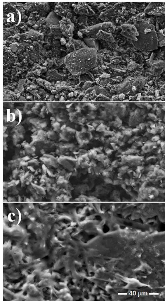
**Figure 2.** FESEM images for the systems (a) Gr, (b) Gr/IL and (c) Gr/IL/Co. Magnification = 2500 $\times$ .
