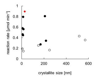
**Figure 1.** Photocatalytic activity of commercial titania samples for oxidative decomposition of acetic acid under UV/vis irradiation (Usually smaller crystallite size and anatase presence result in high photocatalytic activity.); P25—red rhombus ( $\blacklozenge$ ); anatase-rich samples—solid circles ( $\bullet$ ); rutile-rich samples—empty circles ( $\bigcirc$ ); reaction rate—rate of CO<sub>2</sub> evolution.
