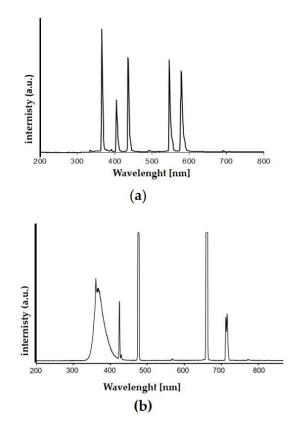
**Figure 5.** Emission spectra of UV/vis lamps used for the investigation of titania photoactivity on: (a) Oxidative decomposition of acetic acid, and (b) human breast cancer cells.
