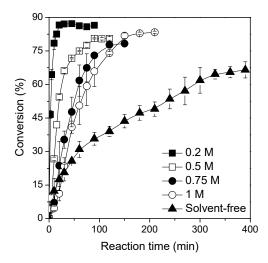
**Figure 4.** Effect of reactants concentration and organic solvent on the ester synthesis. The reactions were performed at 56 °C, 240 rpm, acid:alcohol molar ratio 1:3, and biocatalyst concentration of 800 U of activity by using TLL–Octyl–SiO<sub>2</sub> as biocatalyst.
