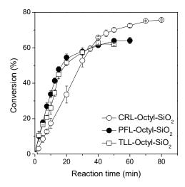
**Figure 1.** Effect of lipase source on the ester synthesis course. The reactions were performed at 40 °C, 240 rpm, stoichiometric acid:alcohol molar ratio containing 0.2 M of palmitic acid in heptane medium and biocatalyst concentration of 300 units of hydrolytic activity (U).
