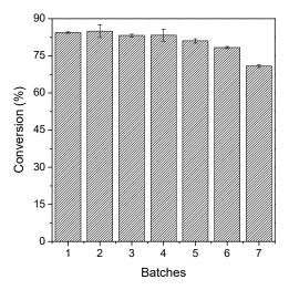
**Figure 6.** Reusability tests of TLL–Octyl–SiO $_2$  after seven consecutive batches of ester synthesis of each 150 min each in a heptane medium. The reactions were performed at 56 °C, 240 rpm, acid:alcohol molar ratio 1:3, and biocatalyst concentration of 800 U.
