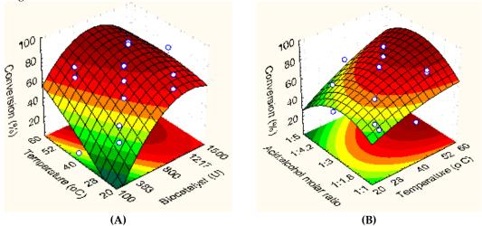
**Figure 3.** 3D surface and contour plots for ester synthesis. – Effect of biocatalyst concentration and reaction temperature **(A)**; and acid:alcohol molar ratio and reaction temperature **(B)** on the conversion percentage.
