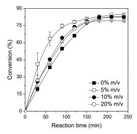
**Figure 5.** Effect of molecular sieves concentration on the ester synthesis. The reactions were performed at 56 °C, 240 rpm, acid:alcohol molar ratio 1:3, and biocatalyst concentration of 800 U of activity by using TLL–Octyl–SiO<sub>2</sub> as biocatalyst.
