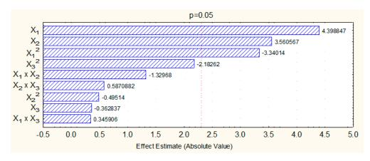
**Figure 2.** Pareto diagram showing the effect of independent parameters biocatalyst concentration  $(x_1)$ , reaction temperature  $(x_2)$ , and acid:alcohol molar ratio  $(x_3)$  and their interactions on the conversion percentage in solketal palmitate synthesis.
