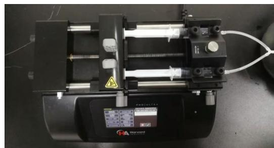
**Figure 1.** Syringe pump and reactant injector.
