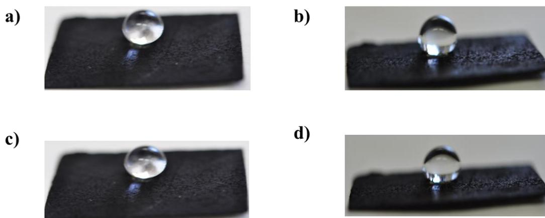
**Figure S1.** Photos of photocathode substrates Sigracet 35BC (on the left) and Sigracet 35BC + FEP 7% (on the right) after 0 s (a, b) and after 1800 s (c, d).
