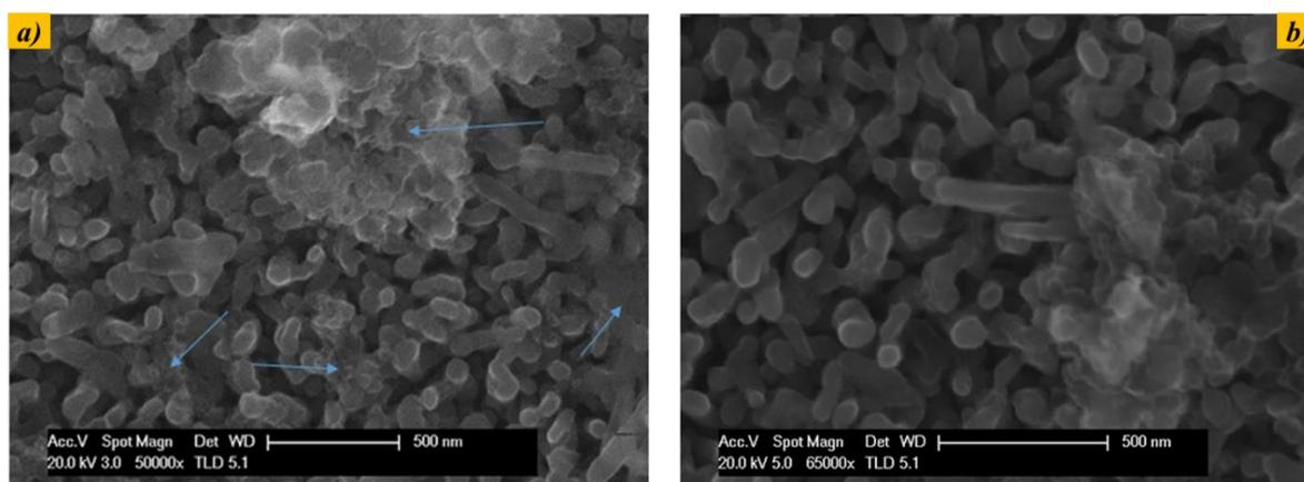
**Figure S8.** SEM images of the outer NiFeO<sub>x</sub>-coated hematite photoanode surface, before (a) and after (b) the durability test.
