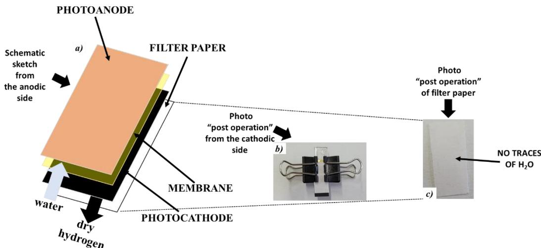
**Figure S6.** Schematic sketch (a) and photograph (b) of the photoelectrochemical cell (PEC) with carbonaceous gas diffusion layer as cathode substrate and filter paper to highlight any traces of water (left); (c) photograph of filter paper “post operation”.
