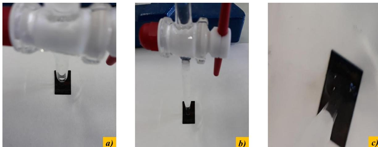
**Figure S7.** Images of a 60 cm water column (about 60 mbar) in a burette placed perpendicular to a CuO/ Sigracet 35BC + FEP 7% sample at the beginning (a), after 1800 s (b), after 15000 s (c).
