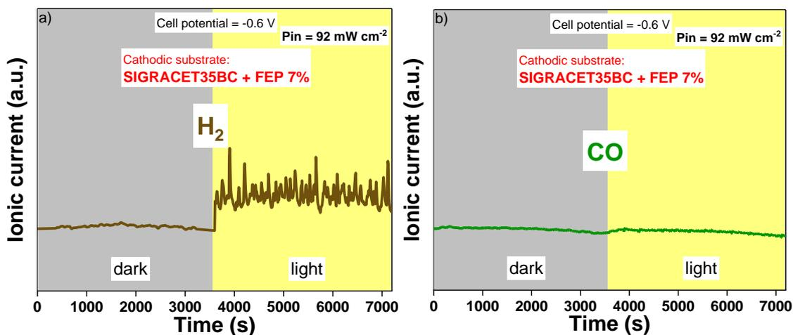
**Figure S5.** Mass spectrometry analysis during potentiostatic test (applied cell bias of -0.6 V) of the PEC cell (glass+FTO+Fe<sub>2</sub>O<sub>3</sub>+NiFeO<sub>x</sub>+ionomer/FAA-3/ionomer+CuO+ Sigracet 35BC+FEP7%): H<sub>2</sub> ionic current (a) and CO ionic current (b).
