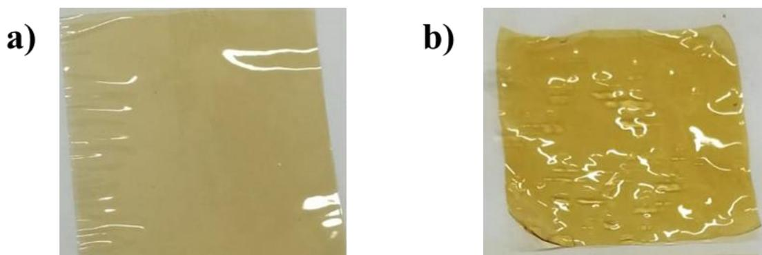
**Figure S4.** Photographs of transparent anionic membrane FAA-3 either dry (a) or wet (b).
