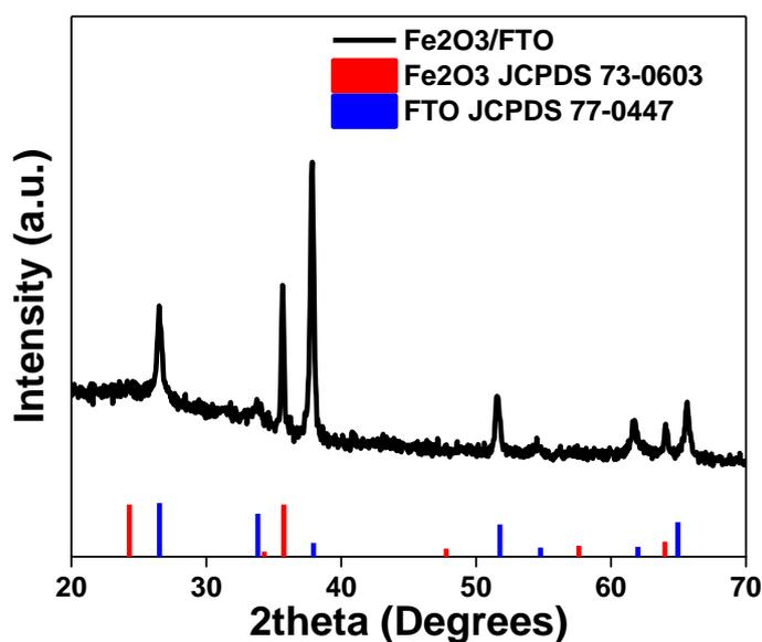
**Figure S2.** XRD pattern of synthesized anodic semiconductor  $\text{Fe}_2\text{O}_3$  deposited on FTO glass and relative JCPDS cards.
