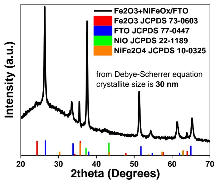
**Figure S3.** XRD pattern of synthesized anodic semiconductor  $\text{Fe}_2\text{O}_3 + \text{NiFeOx}$  deposited on FTO glass and relative JCPDS cards.
