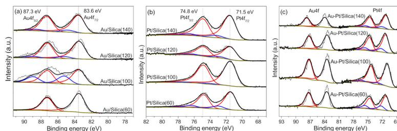
**Figure 5.** XPS spectra of (a) Au 4f of a series of Au/silica; (b) Pt 4f of a series of Pt/silica; (c) Au 4f and Pt 4f of a series of Au-Pt/silica.
