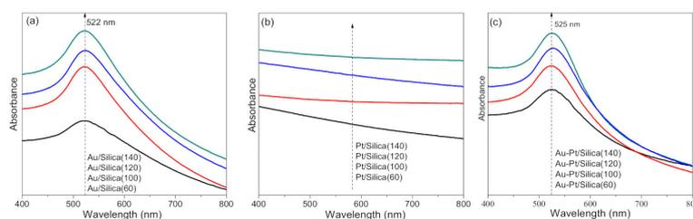
**Figure 2.** UV-Vis spectra of three series of catalysts of (a) Au/silica, (b) Pt/silica, and (c) Au-Pt/silica.
