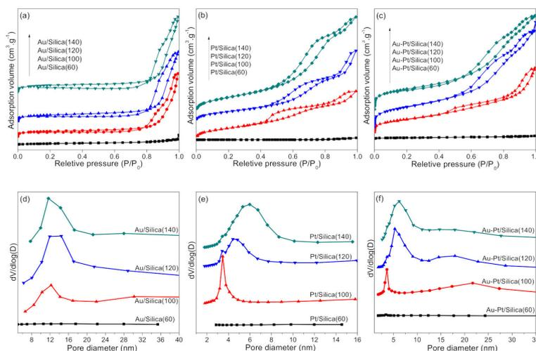
**Figure 3.** N<sub>2</sub> adsorption-desorption isotherms of (a) Au/silica, (b) Pt/silica, and (c) Au-Pt/silica; BJH pore size distribution of (d) Au/silica, (e) Pt/silica, and (f) Au-Pt/silica.
