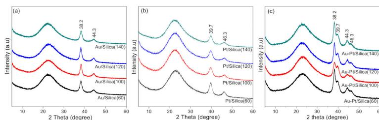
**Figure 1.** Powder XRD patterns of as-made three series of catalysts of (a) Au/silica, (b) Pt/silica, and (c) Au-Pt/silica.
