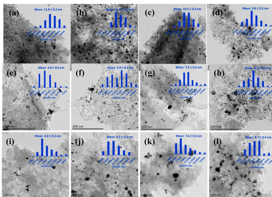
**Figure 4.** TEM images of (a) Au/silica(60), (b) Au/silica(100), (c) Au/silica(120) and (d) Au/silica(140); (e) Pt/silica(60), (f) Pt/silica(100), (g) Pt/silica(120) and (h) Pt/silica(140); (i) Au-Pt/silica(60), (j) Au-Pt/silica(100), (k) Au-Pt/silica(120) and (l) Au-Pt/silica(140). Insets are histograms of metal particle size distribution.
