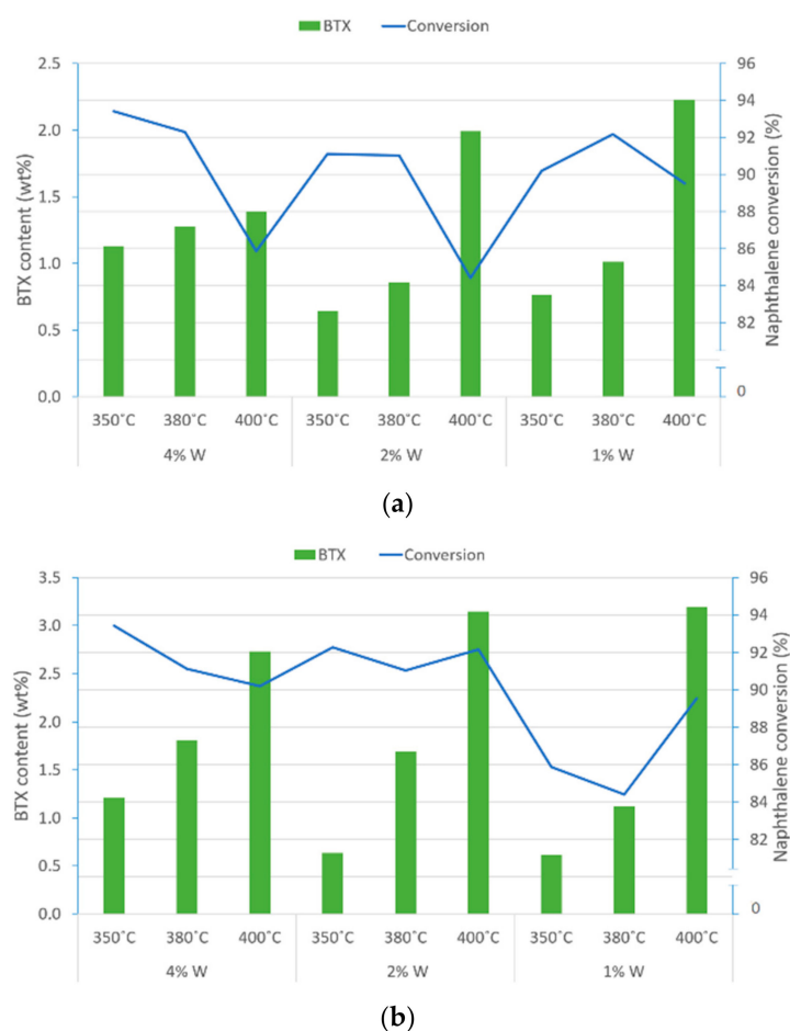
Figure 1. Naphthalene conversion versus tungsten molar ratio and reaction temperature, and benzene, toluene, and xylene (BTX) selectivity with (a) NiWS-HY(0.5%), (b) NiWS-HY(1%) catalysts at standard conditions P = 5 MPa, t = 5 h, and W:Ni ratio = 1:2.
