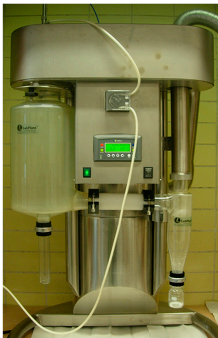
Figure S5. The Lab-Plant SD-06 Laboratory Spray Dryer
