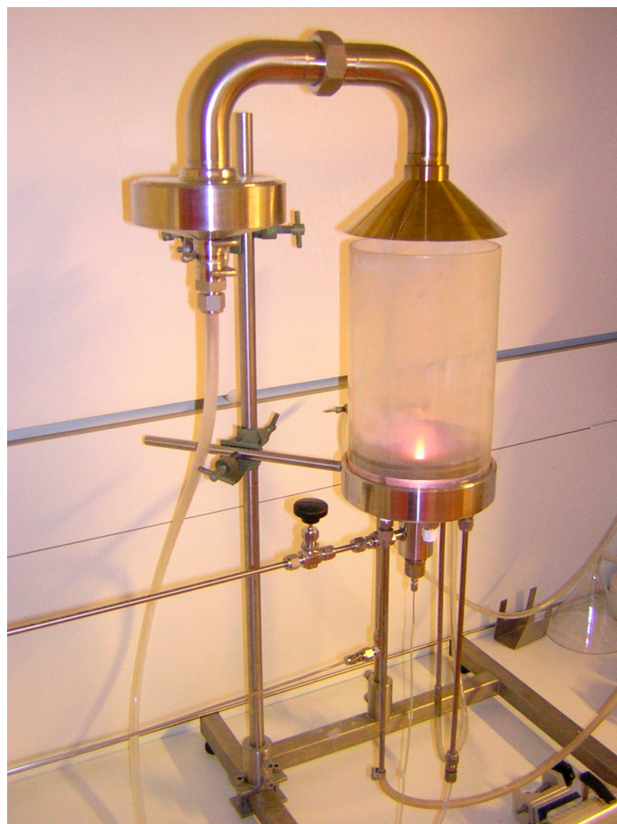
Figure S3. The setup for flame spray pyrolysis employed at DTU
