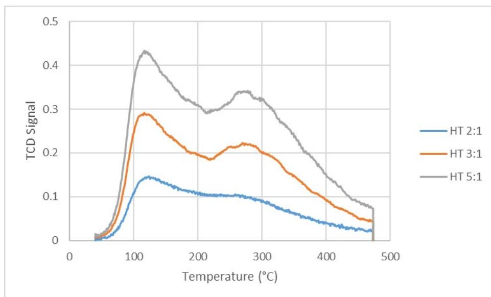
Figure S1 – TPD-CO<sub>2</sub> of hydrotalcite samples.
