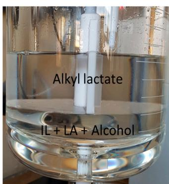
**Scheme 4.** Photograph of the reactor with the postreaction mixture of model esterification of lactic acid with 2-ethylhexanol (IL—ionic liquid).
