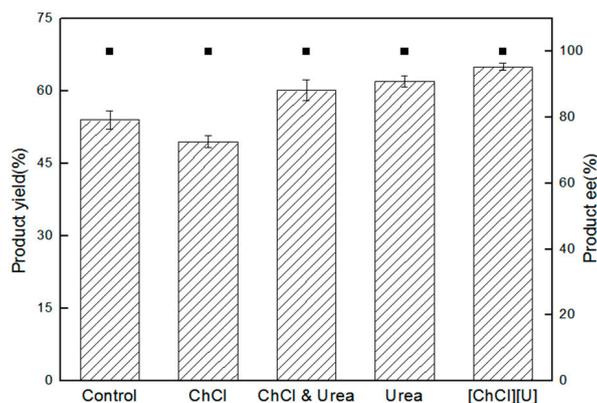
**Figure 3.** Effect of [ChCl][U] components on the bioreduction of BTAP to BTPE catalyzed by *R. erythropolis* XS1012. Reaction conditions: 9 mL buffer ( $\text{Na}_2\text{HPO}_4$ - $\text{NaH}_2\text{PO}_4$ , 100 mM, pH 7.0), 45 g (DCW)/L *R. erythropolis* XS1012, 150 mM BTAP, 50 g/L glucose, 10% (*v/v*) isopropanol content, 30 °C and 200 rpm for 24 h. 1% *w/v* ChCl&U, ChCl and Urea were added according to the content of 1% *w/v* [ChCl][U](1:1).
