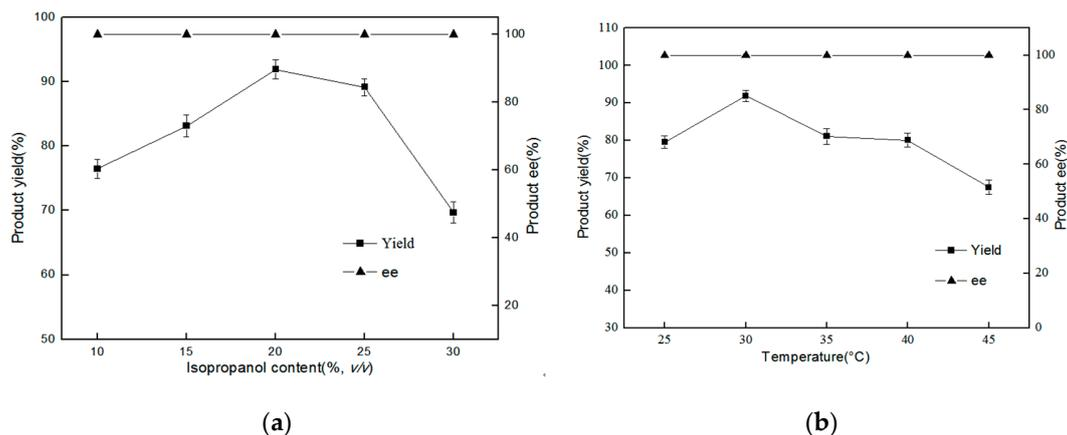
**Figure 5.** Effects of isopropanol content (a), reaction temperature (b) on the asymmetric reduction of BTAP. Reaction conditions: phosphate buffer ( $K_2HPO_4$ - $KH_2PO_4$ , 100 mM, pH 6.5),  $[ChCl][U](1:1)$  1% (w/v), 45 g (DCW)/L *R. erythropolis* XS1012, isopropanol content (20%, v/v) (b), 150 mM BTAP, 30°C (a) and 200 rpm for 24 h.
