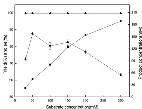
**Figure 1.** Effect of substrate concentration on the asymmetric reduction of BTAP in the phosphate buffer system. Symbols: (●) yield and (▲) e.e.; (■) product concentration. Reaction conditions: phosphate buffer ( $\text{Na}_2\text{HPO}_4$ - $\text{NaH}_2\text{PO}_4$ , 100 mM, pH 7.0), 45 g (DCW)/L *R. erythropolis* XS1012, 50 g/L glucose, 15% (*v/v*) isopropanol content, various BTAP concentration, and 30 °C, 200 rpm for 24 h.
