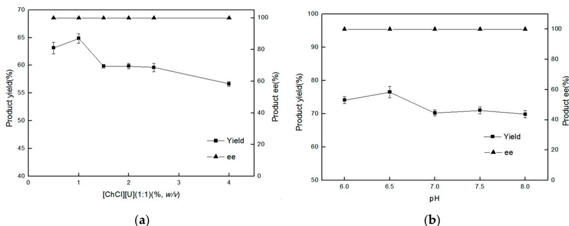
**Figure 4.** Effect of [ChCl][U](1:1) content (a), pH (b) on the asymmetric reduction of BTAP. Reaction conditions: 9 mL phosphate buffer (100 mM, pH 7.0) (a), various (*w/v*) [ChCl][U](1:1) (a), various pH of  $\text{K}_2\text{HPO}_4$ - $\text{KH}_2\text{PO}_4$  buffer (b), 1% (*w/v*) [ChCl][U](1:1) (b), 45 g (DCW)/L *R. erythropolis* XS1012, 1 mL isopropanol (10%, *v/v*), 50 g/L glucose, 150 mM BTAP, 30 °C and 200 rpm for 24 h.
