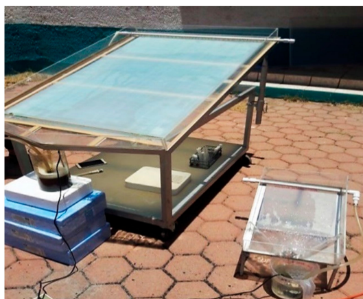
Figure 7. Solar reactors with 1 \text{ m}^2 (left) and 1/10 \text{ m}^2 contact surface (right).
