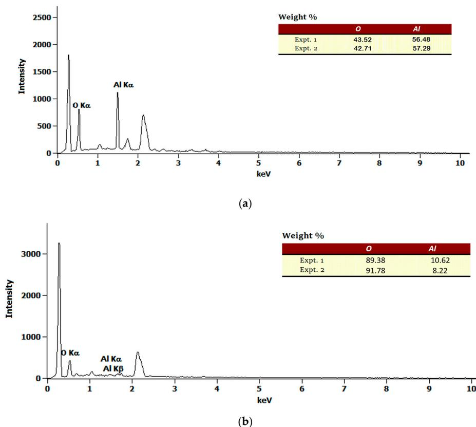
**Figure 4.** (a) energy dispersive X-ray (EDX) spectra of  $\text{Al}_2\text{O}_3$  nanoparticles and (b) EDX spectra of PVA- $\text{Al}_2\text{O}_3$  (10 wt%).
