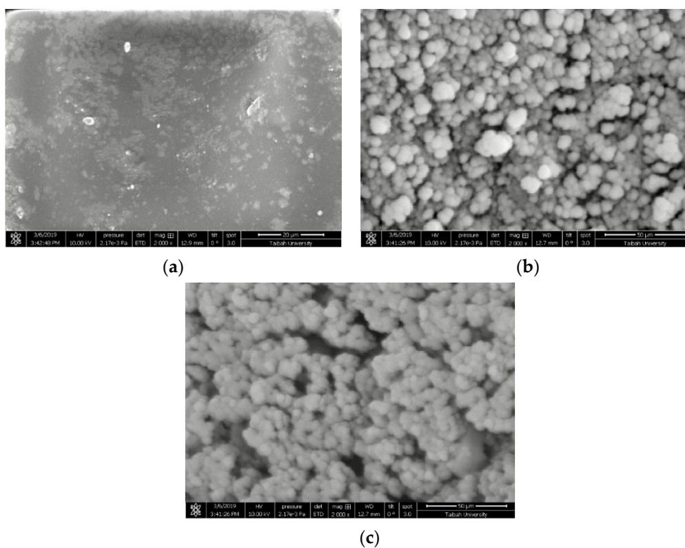
**Figure 3.** (a) SEM image of PVA; (b) SEM image of  $\text{Al}_2\text{O}_3$  nanoparticles; and (c) SEM image of PVA/ $\text{Al}_2\text{O}_3$  film.
