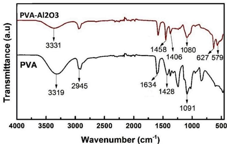
Figure 2. FTIR of original PVA and PVA-Al<sub>2</sub>O<sub>3</sub> (10 wt%) nanocomposite.
