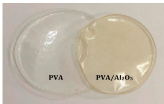
**Figure 6.** Images of virgin PVA and PVA-Al<sub>2</sub>O<sub>3</sub> nanocomposite.
