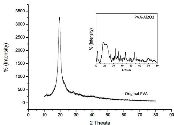
**Figure 5.** XRD pattern of virgin PVA and PVA- $\text{Al}_2\text{O}_3$  nanocomposite.
