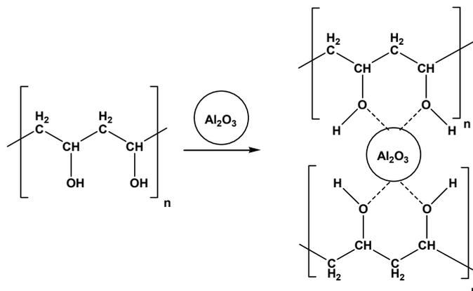
Figure 1. Structure of a PVA-Al<sub>2</sub>O<sub>3</sub> nanocomposite.
