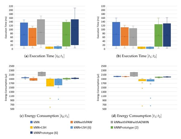
**Figure 9.** Energy Consumption ( $\mu$ J) and Execution Time (ms) (per instance) of the various *k*NN methods for the *PAMAP2* dataset.
