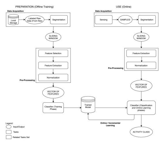
**Figure 1.** Block diagram of the Human Activity Recognition (HAR) system considered. In the case of *k*NN prototypes the Trained Model is a storage of instances.
