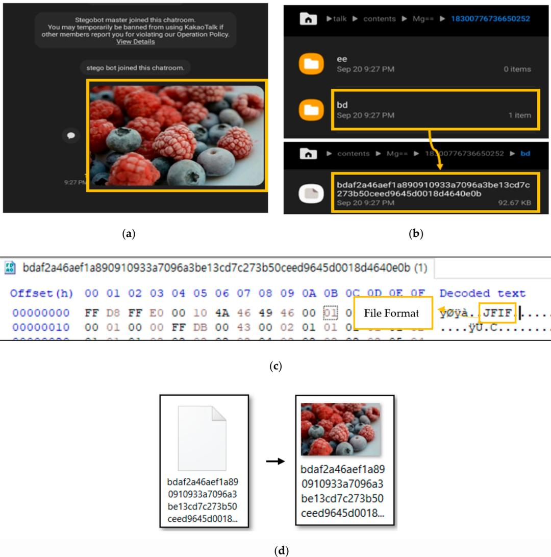
**Figure 5.** Locating an image file downloaded from a KakaoTalk chatroom at the smartphone. (a) Defender clicks on the uploaded image. (b) Location of downloaded image files. (c) Hex view of Stegano image file. (d) An example of converting a file without an extension into an image file.
