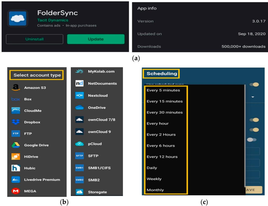
**Figure 6.** Implementation of automated collection component. (a) Freeware sync applications FolderSync. (b) Synchronization method selection function. (c) Periodic file transfer function.
