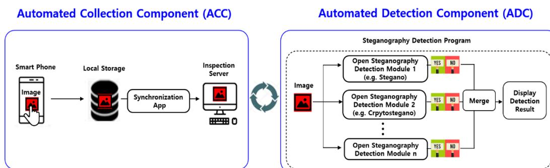
**Figure 4.** Design of our proposed system with two main components (automated collection component and automated detection component).
