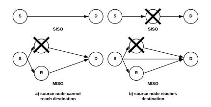
Figure 4. Single-in-single-out vs. Multi-in-single-out (CC) with a corrupt relay node.
