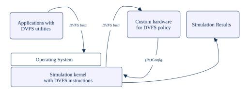
Figure 1. Hardware-assisted DVFS simulation mechanism proposed by [3].
