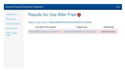
**Figure 6.** Report page for use-after-free vulnerabilities found in the project. Clicking on a link in the table of vulnerabilities will display the formatted contents of the file in question.
