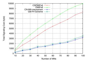
Figure 10. Performance of signalling cost vs. the number of MNs (CN-MN mechanism).
