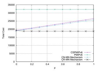
Figure 8. The overall TC of inter-cluster operation for CR-MN mechanism.
