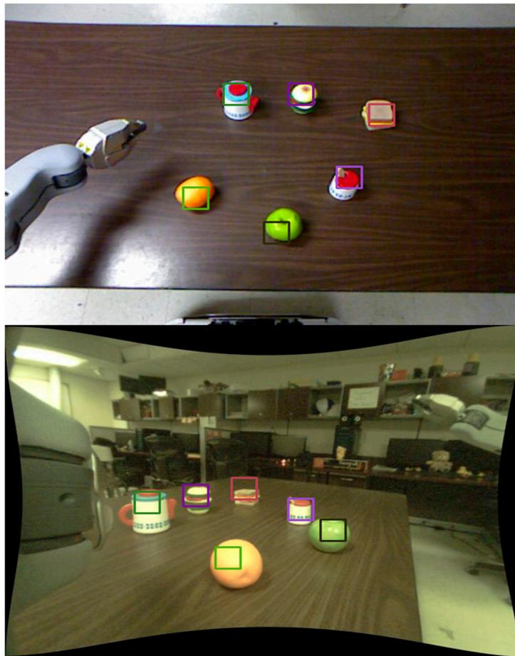
Figure 5. Examples of object matching in a test table-top situation. Bounding boxes with the same color are matched in the main view (Top image) and the secondary view (Bottom image).
