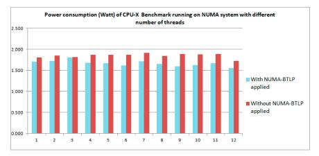
**Figure 2.** Power consumption of CPU-X Benchmark running on NUMA system with different number of threads which is set statically, when NUMA-BTLP algorithm [5] is applied and when the algorithm is not applied at compile-time.
