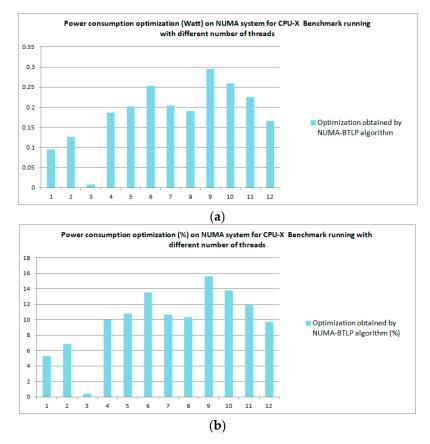
**Figure 3.** Power consumption optimization obtained on NUMA system for CPU-X Benchmark running with different number of threads which are set statically: (a) Optimization expressed in Watt (b) Optimization expressed in %. NUMA-BTLP: Non-Uniform Memory Access—Balanced Task and Loop Parallelism.
