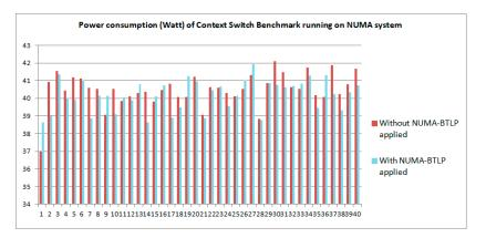
**Figure 4.** Power consumption (Watt) for Context Switch Benchmark, obtained on 40 runningrounds of the application on NUMA system, both when NUMA-BTLP algorithm is applied at compile-time and when the algorithm is not applied.
