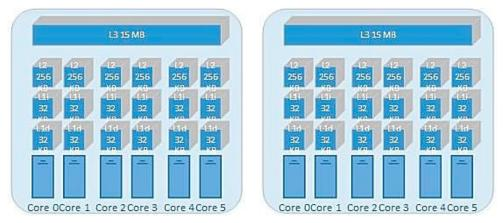
Figure 1. Intel Xeon E5-2630 v2 sockets (CPUs) of Fujitsu Workstation Celsius r930 power.
