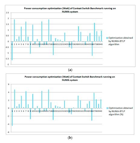
**Figure 5.** Power consumption optimization per round for Context Switch Benchmark running 40 times on NUMA system: (a) Optimization expressed in Watt (b) Optimization expressed in %.
