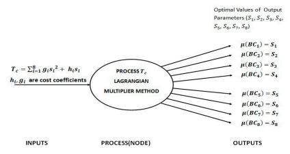
**Figure 5.** Data flow graph (DFG) of process T<sub>c</sub> (Lagrangian multiplier method).
