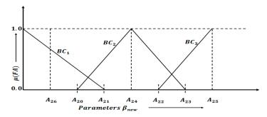
**Figure 6.** Fuzzy Set A used for computing fuzzy membership in process T<sub>c</sub>.
