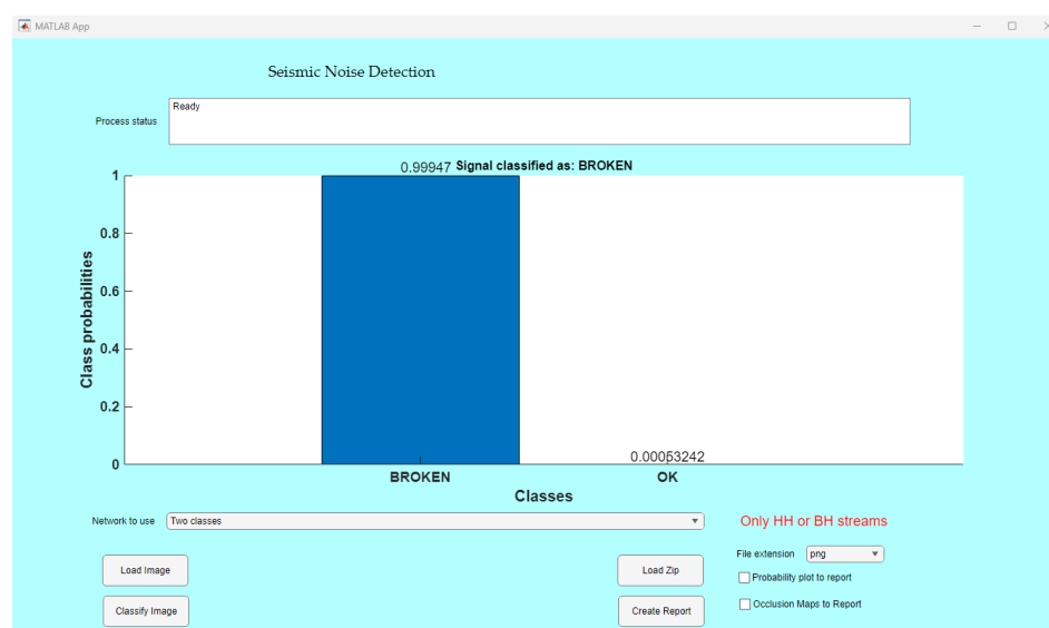
Figure 4. Result of a two-class neural network for IV.TERO–HHZ. The bar plot shows that the station belongs to the class BROKEN with probability higher than 99%, and it belongs to class OK with probability lower than 1%. The predicted label, here BROKEN, is written on the top of the plot.
