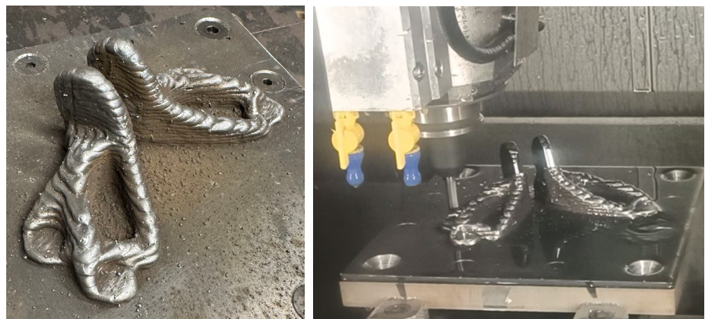
Figure 12. Final part after WAAM process before milling (left) and while milling (right).
