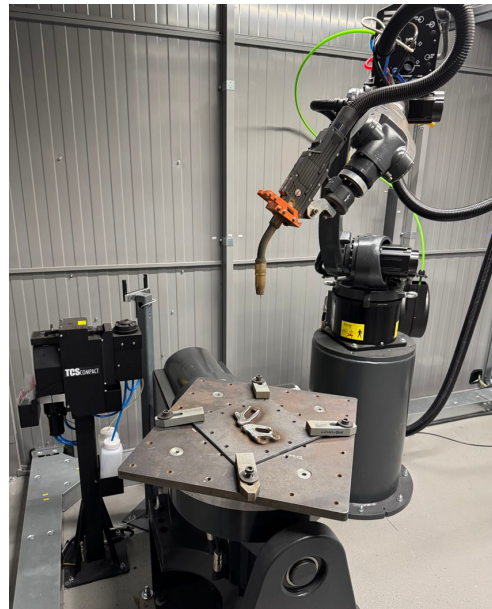
Figure 3. Robotic cell setup for WAAM.
