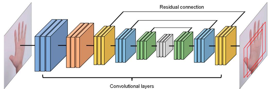
**Figure 2.** Architecture of the palm detector. The palm detector can easily detect palm regions with a relatively fixed shape. The hand area can be obtained by expanding the palm area. The hourglass-like shape of the model structure helps to detect hands of different scales.
