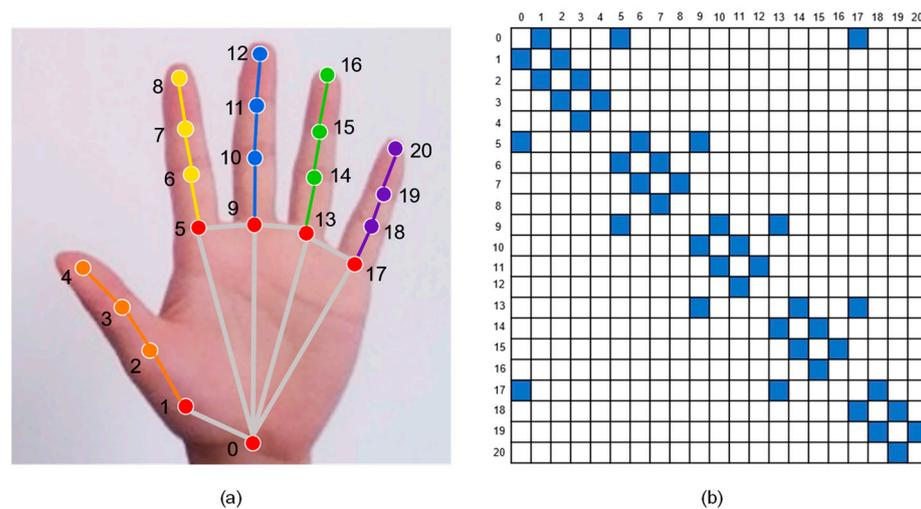
**Figure 5.** (a) Hand landmarks extracted by the model are spatially interconnected to form a skeletal map of hand. (b) Adjacency matrix of 21 hand landmarks.
