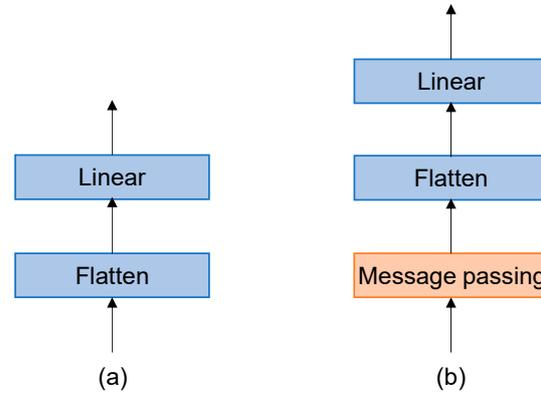
**Figure 4.** (a) Common MLP classification head. (b) MLP classification head embedded in the message passing layer called GMLP. GMLP first passes the message based on the adjacency matrix between the hand joints to preserve some of the spatial features and then flattens them to obtain the output vectors through a linear layer.
