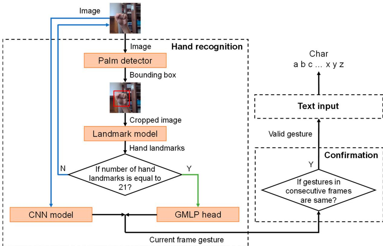
**Figure 1.** Pipeline of the proposed hand recognition-based text input method called iHand. The hand recognition module outputs class label. The gesture confirmation module detects whether the gesture is valid. The text input module is responsible for entering letters.
