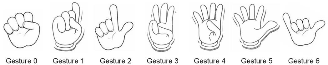
**Figure 8.** Seven hand gestures used to input letters. Gesture x can select xth row or xth column of the character layout.
