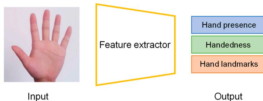
**Figure 3.** Pipeline of hand landmark model. The input is a picture, and the model has three outputs sharing a feature extractor: hand presence, handedness, and hand landmarks.
