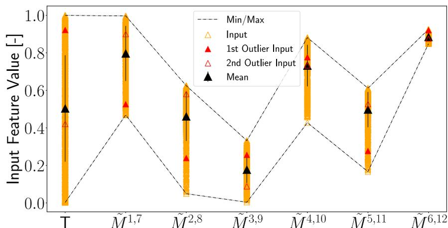
**Figure 25.** Feature input values artificially generated for damage case D16 are plotted. Shown are the mean value together with the standard deviation, as well as the minimum and maximum values of the input. The inputs for the first and second outliers, highlighted in Figure 18d, are plotted in a similar manner as in Figure 18d.
