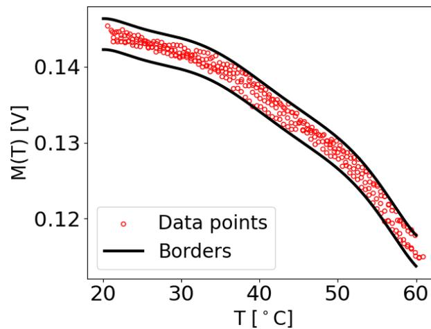
**Figure 5.** Examples of  $M$  values extracted from the original data of the OGW dataset, which were used to establish the borders from the maximum function  $M^{i,j}(T)$ , specifically for the damage-free measurement for the case where  $i = 1$  and  $j = 7$ .
