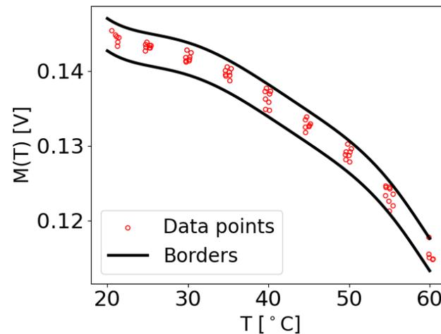
**Figure 14.** Examples of  $M$  values extracted for  $T = 20, 25, 30, 35, 40, 45, 50, 55, 60$  °C, which were used to establish the borders from the maximum function  $M^{i,j}(T)$ , specifically for the damage-free measurement for the case where  $i = 1$  and  $j = 7$ .
