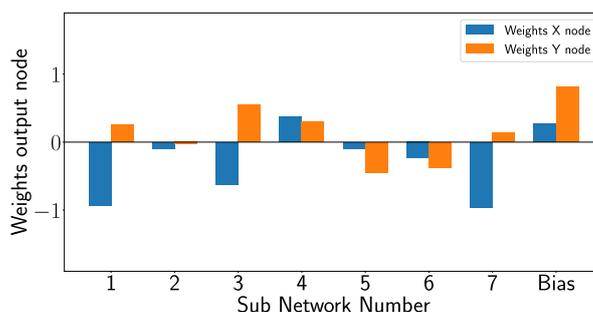
**Figure 23.** Weights of the output nodes, where the x node is responsible for predicting the x-position of the damage, and the y node is responsible for predicting the y-position of the damage.
