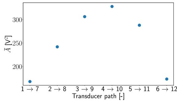
**Figure 6.** Average values of the area under the envelope  $\bar{A}^{i,j}$  for different transducer paths for the damage-free case.
