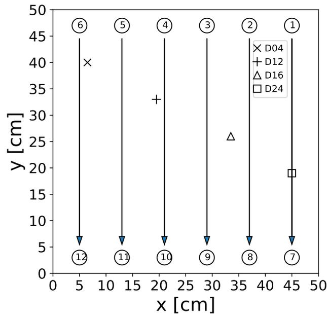
**Figure 2.** Sketch of the CFRP plate used for UGW measurements. The circles with numbers represent the transducer positions; numbers correspond to the transducer indices. The arrows show the transducer paths used in this study. While the D04 (x), D12 (+), D16 (△), and D24 (□) markers correspond to the position of the artificial damage applied to the surface of the plate.
