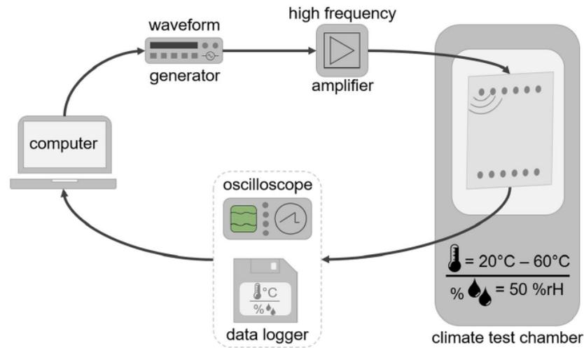
**Figure 3.** A sketch of the experimental setup utilized for the UGW measurements. The image is sourced from [27] under the Creative Commons Attribution 4.0 International License (<http://creativecommons.org/licenses/by/4.0/> (accessed on 10 January 2024)).
