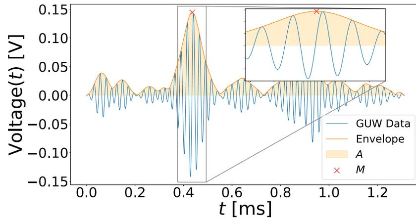
**Figure 4.** Example for maximum  $M$  and area under the envelope  $A$  extraction from a UGW signal. The displayed signal was recorded at sensor path 1  $\rightarrow$  7 with a frequency of 40 kHz at a temperature of 20 °C.
