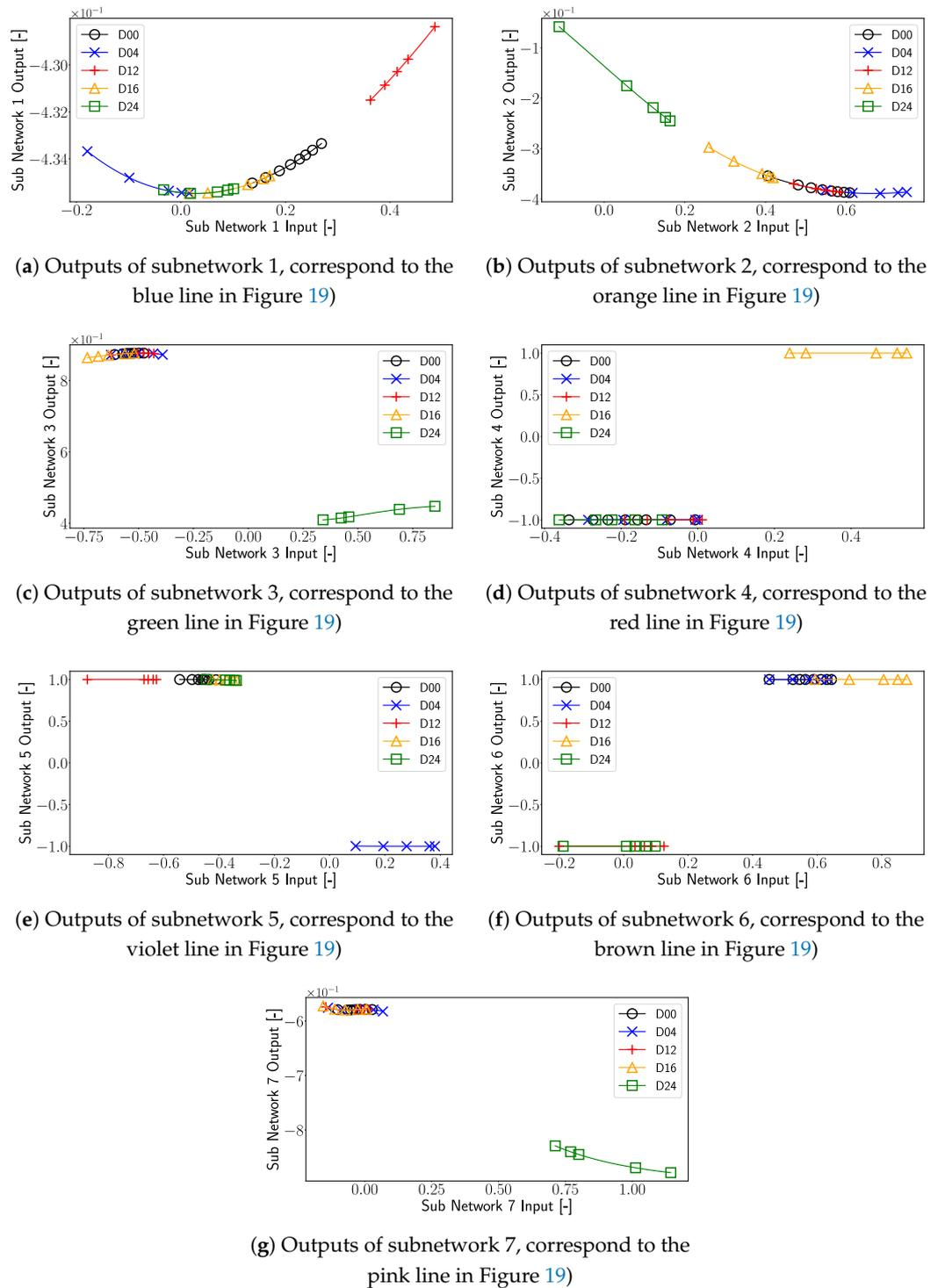
**Figure 20.** Outputs of the sub networks as a function of the original data as input. The markers used in the plot correspond to different damage cases of the plate, with D00 representing the damage-free case. In the interest of visibility for every damage case dataset, a marker was placed at the minimum and maximum data points, as well as at every 200th data point within these boundaries.
