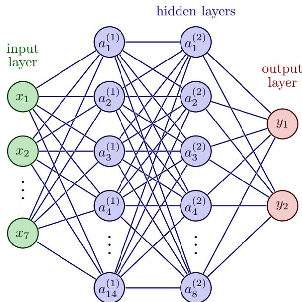
**Figure 7.** Sketch of the used classical fully connected ANN architecture. The architecture consisted of input nodes denoted as  $x$ , where  $x_1 = \tilde{T}$ ,  $x_2 = \tilde{M}^{1,7}(T)$ , ..., and  $x_7 = \tilde{M}^{6,12}(T)$ . The hidden layers were represented by nodes denoted as  $a$ , and the output layer was denoted as  $y$ .
