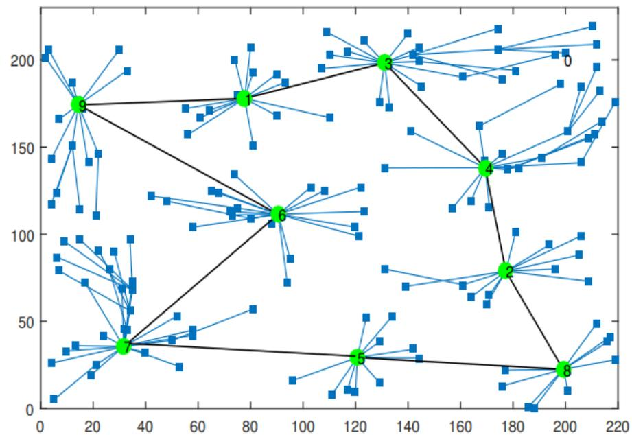
**Figure 4.** DBRkM Run-Time Simulation (average hop count = 1.24, tour length = 1034 m fixed at all rounds).
