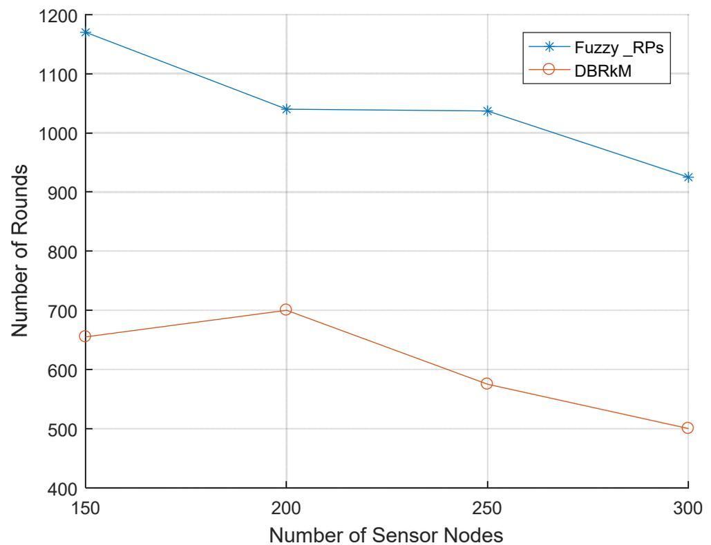
**Figure 9.** Network lifetime vs. number of sensor nodes.
