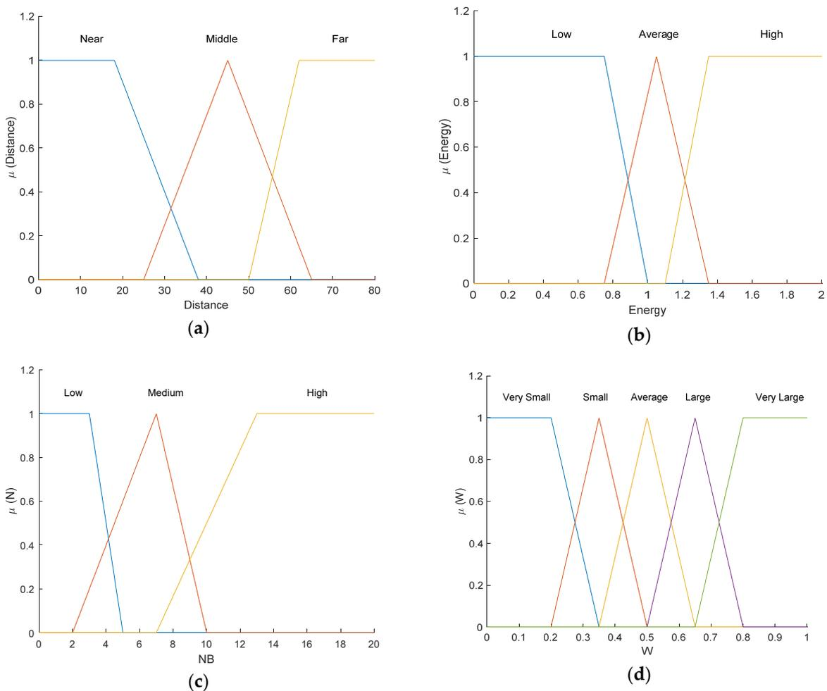
**Figure 3.** Membership functions of the inputs and output. (a) Membership functions of input Distance. (b) Membership functions of input Energy. (c) Membership functions of input (NB). (d) Membership functions of output  $w$ .
