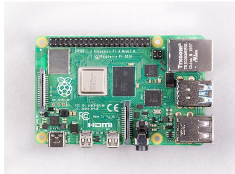
**Figure 1.** Raspberry Pi4 Model B board peripheral device layout. Detailing position of Broadcom BCM2711 processor, RAM, USB Type-C power supply, and network ports. Source: [80].
