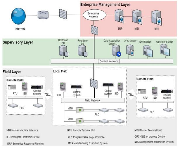
Figure 6. Industrial control system (ICS) network architecture.
