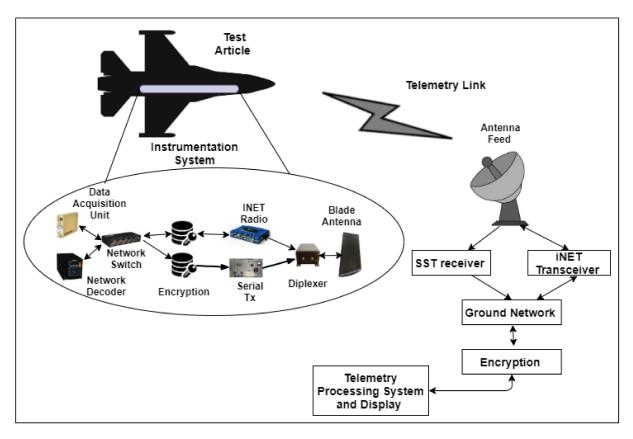
Figure 1. Telemetry network instrumentation and a test article aircraft [4].
