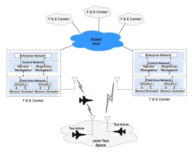
Figure 7. General telemetry architecture.
