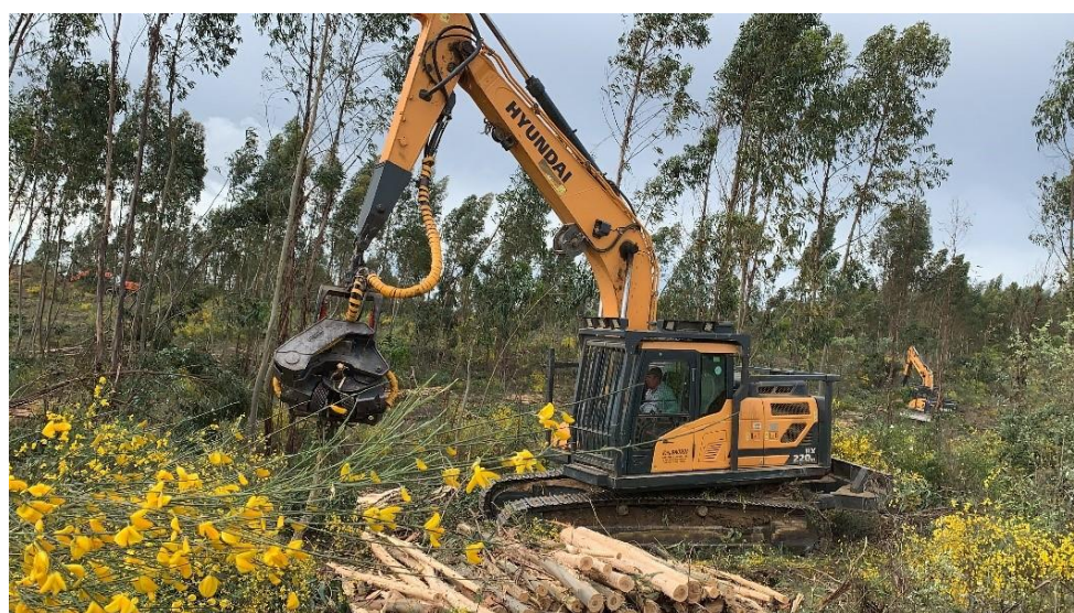
Figure 1. Harvester machine in operation equipped with a processor head.
