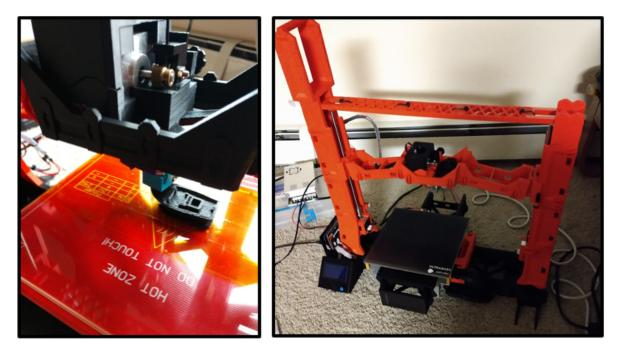
Figure 4. Conceptual Prototype of a 3D-printed 3D print-capable robot. The left image shows an in-progress 3D print.
