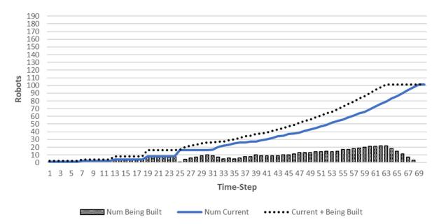
Figure 11. Robot build rate of the decentralized homogeneous (DHO) configuration on experimental condition A0.
