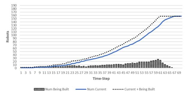
Figure 13. Robot build rate of the hierarchical homogeneous (HHO) configuration on experimental condition A0.
