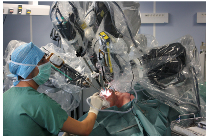
Figure 1. Robot arms introduced transorally during oropharynx surgery.
