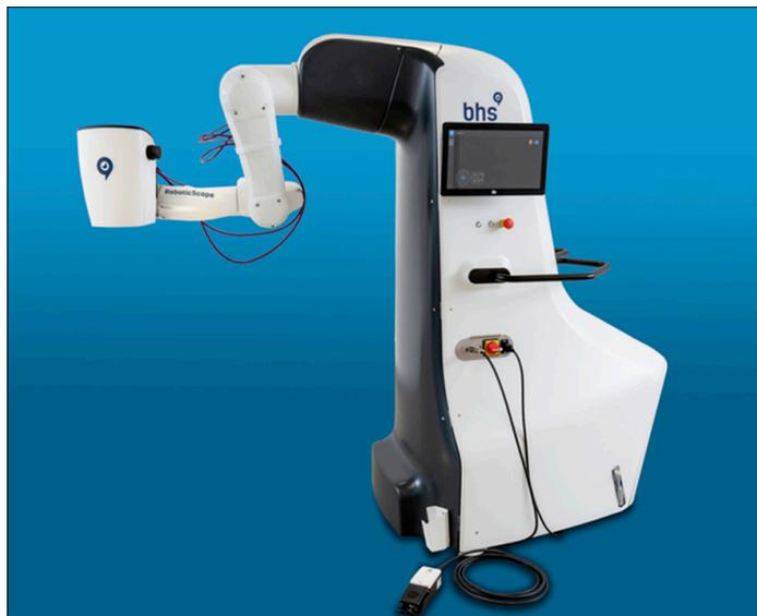
**Figure 4.** RoboticScope<sup>®</sup>-system with a high-resolution 3D-camera and a head-mounted display. Reproduced with kind permission from BHS Technologies<sup>®</sup>, Innsbruck, Austria, © 2020.
