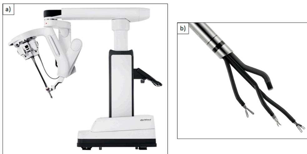
**Figure 3.** (a) DaVinci Single-Port (SP)<sup>®</sup> robotic system; (b) Single 2.5 cm cannula containing three instrument arms and an endoscope. Reproduced with kind permission from Intuitive Surgical<sup>®</sup>, Inc., Sunnyvale, CA, USA, © 2021.
