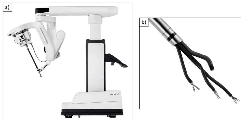
Figure 3. (a) DaVinci Single-Port (SP) ® robotic system; (b) Single 2.5 cm cannula containing three instrument arms and an endoscope. Reproduced with kind permission from Intuitive Surgical ® , Inc., Sunnyvale, CA, USA, © 2021.
