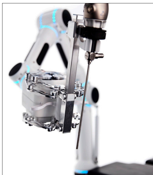
Figure 6. Cirq®. Robot-assisted endoscope guidance system with a mechatronic arm consisting of several segments with 7 degrees of freedom and the possibility to attach a conventional endoscope. Reproduced with kind permission from Medineering/Brainlab®, Munich, Germany, © 2021.
