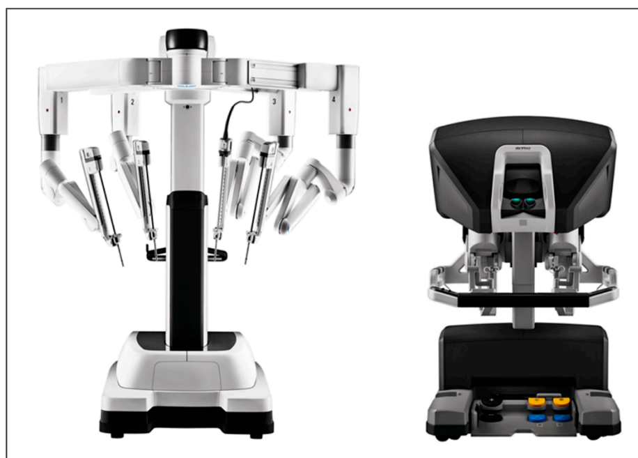
Figure 1. DaVinci Xi®. Multi-port robotic system with camera arm and several working arms for the use of different surgical instruments. Reproduced with kind permission from Intuitive Surgical®, Inc., Sunnyvale, CA, USA, © 2021.
