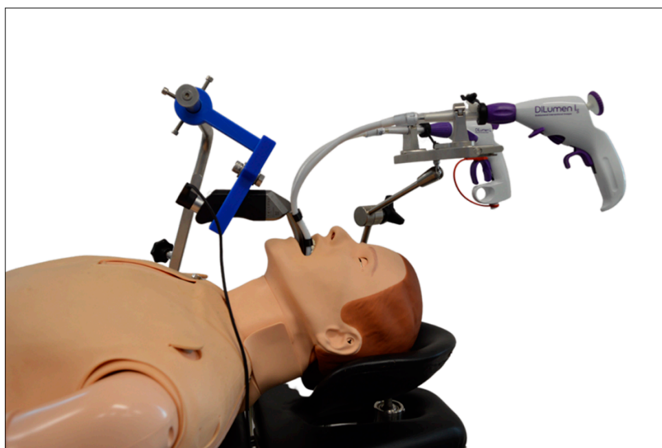
Figure 5. Curved prototype of a video laryngoscope equipped with flexible instruments for laryngeal surgery. Reproduced with kind permission from Schuler et. al., Ulm University Medical Center, Ulm, Germany, © 2021.
