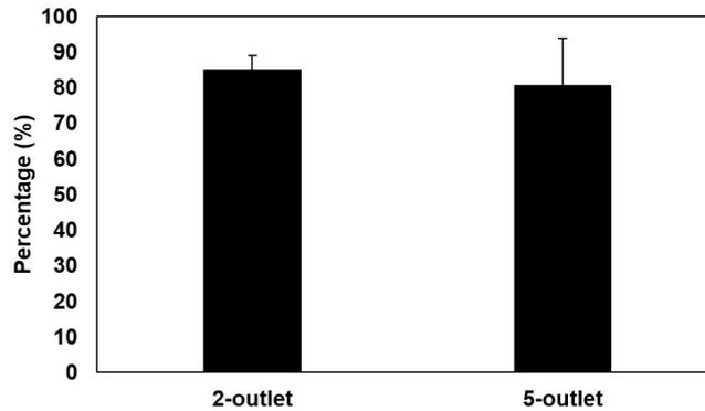
**Figure S1.** The recovery rate of EBCCs in the various versions of the sorting device. The dotted line serves as a reference to the recovery rate of current techniques of EBCC capture.
