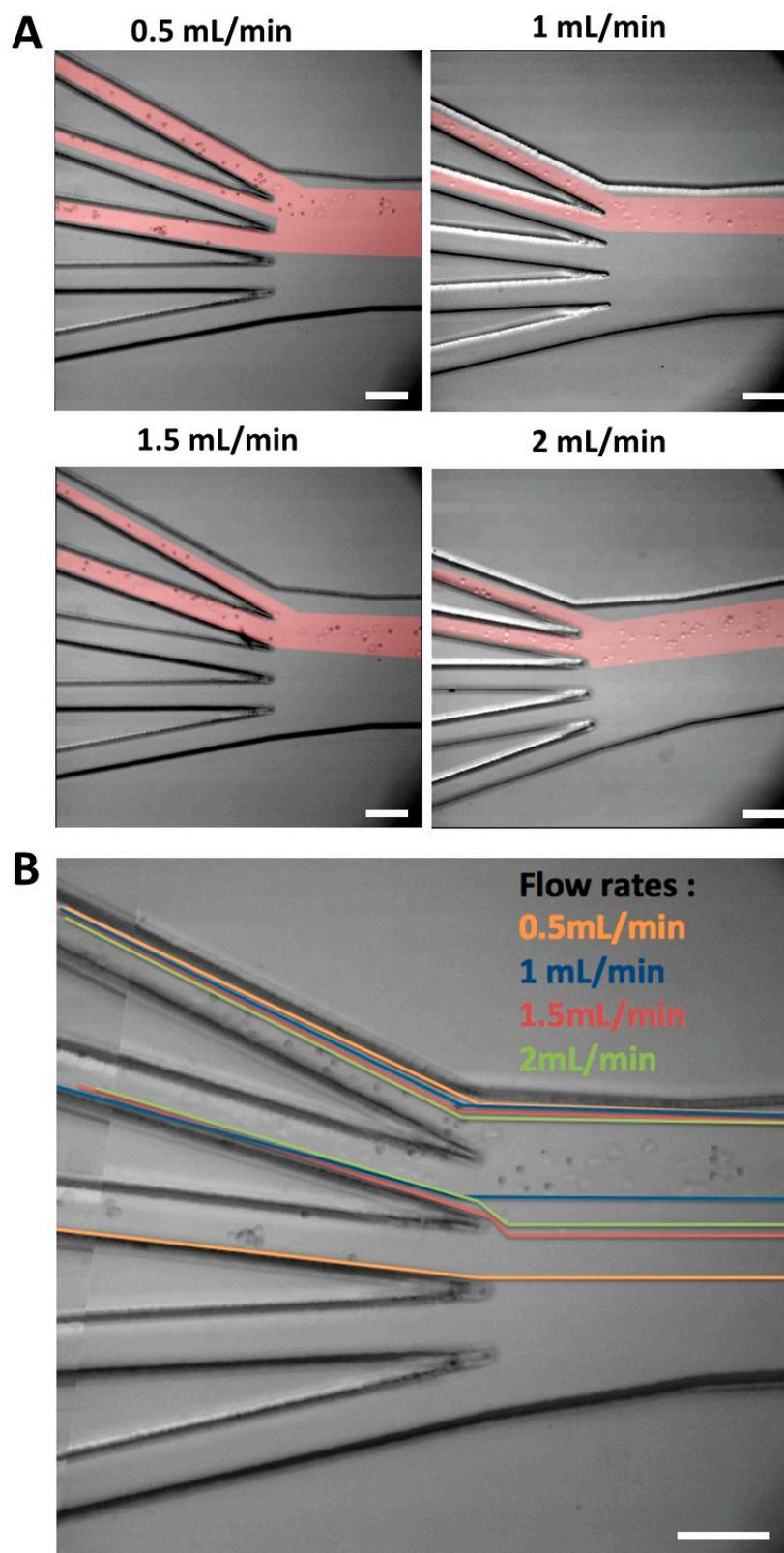
**Figure S3.** Flow rate experiment. (A) 4 flow rates were tested between 1 mL/min and 2 mL/min. (B) Merged cell stream for 4 flow rates. Scale bar is 200  $\mu$ m.
