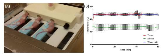
**Figure S6.** Hyperthermia setup. A photo of the hyperthermia setup (**A**) and temperature measurements of tumor (N = 4), mouse (core) (N = 5) and water bath (N = 5) during hyperthermia treatment up to 60 minutes (**B**)
