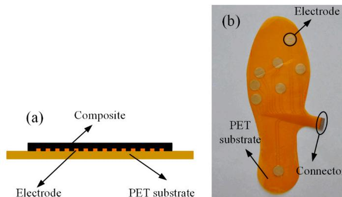
**Figure 7.** (a) Structure diagram of a sensing element (not to scale); (b) fabricated flexible insole with the electrodes and connector.
