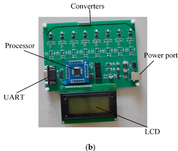
**Figure 8.** (a) Block diagram of the signal processing system; (b) the implemented signal processing system.
