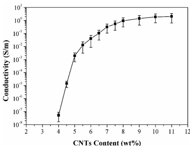
Figure 4. Composite electrical conductivity as a function of MWCNTs content.
