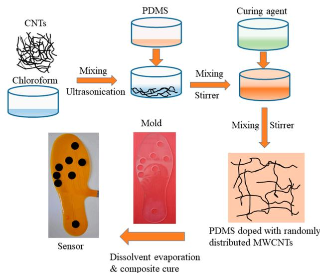
**Figure 1.** Schematic of the processing procedure for preparing a multiwall carbon nanotubes (MWCNTs)/polydimethylsiloxane (PDMS) conductive elastomer and fabricating the plantar pressure sensor.
