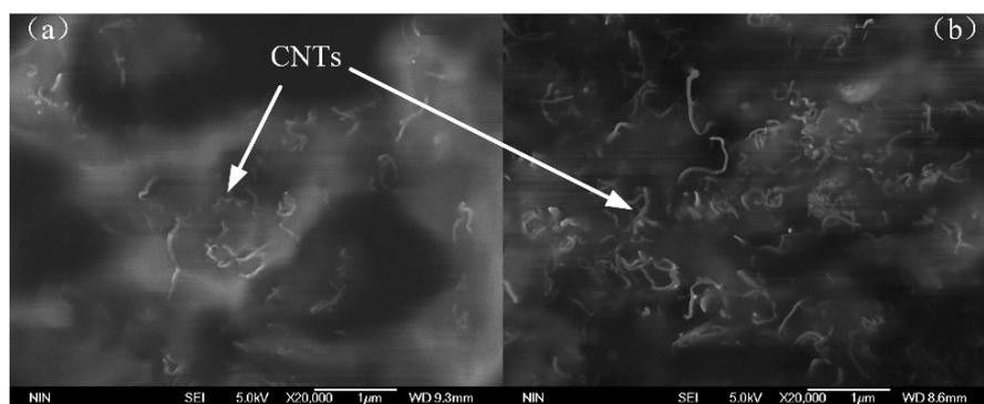
**Figure 3.** (a) Scanning Electron Microscope (SEM) images of the composite with 5 wt% MWCNTs content; (b) SEM images of the composite with 6 wt% MWCNTs content.
