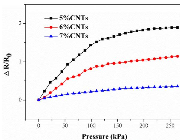
Figure 5. Electromechanical performances composites having different MWCNTs content.
