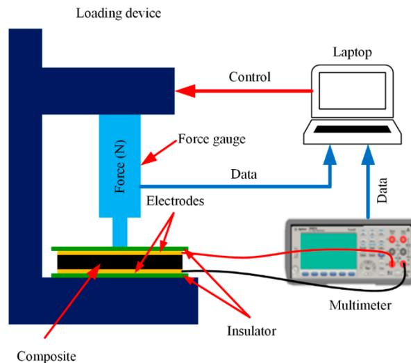
**Figure 2.** Schematic diagram of the experimental setup.
