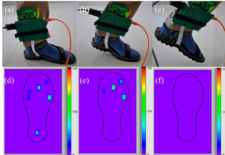
Figure 10. (a) Picture of the foot flat; (b) picture of the heel off; (c) picture of the midswing; (d) plantar pressure of the foot flat; (e) plantar pressure of the heel off; (f) plantar pressure of the midswing.
